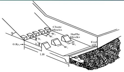
The position of a hydraulic jump below a spillway depends on the spillway head and height, the discharge, the tailwater depth, and the width of the stilling basin.
