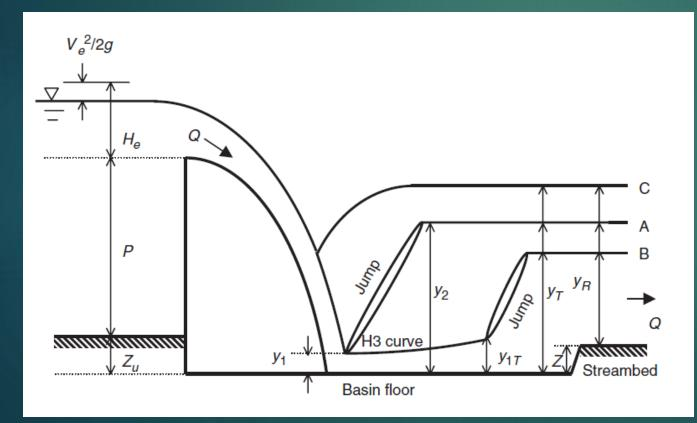
In case A the hydraulic jump occurs at the spillway toe,
