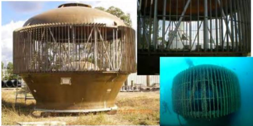
Gold Coast Desalination Plant Intake
