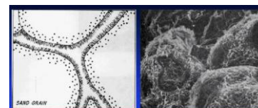
Cause of significant "Clay Bound Water" - detectable with \phi_e From Nissham 1977, SPE 6959
