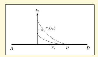
Plate AB initially stationary. Motion with velocity U starts at time t=0
