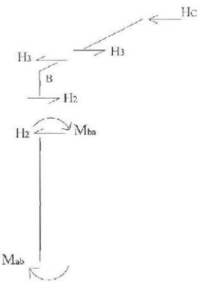
$$H_C = H_3 + 5.4 = H_2 + 5.4 = \frac{M_{AB} + M_{BA}}{6} + 5.4 + 5.4 = \frac{M_{AB} + M_{BA}}{6} + 10.8 \quad (\text{V})$$
