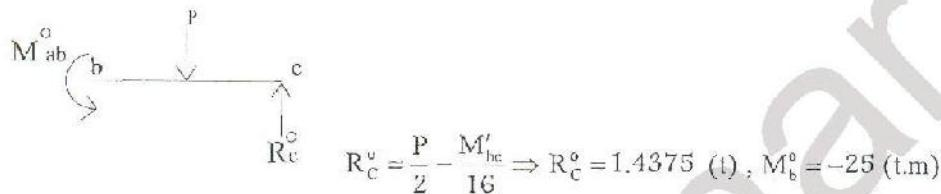
$$R_c^o = \frac{P}{2} - \frac{M'_{bc}}{16} \Rightarrow R_c^o = 1.4375 \text{ (t)} , M_b^o = -25 \text{ (t.m)}$$
