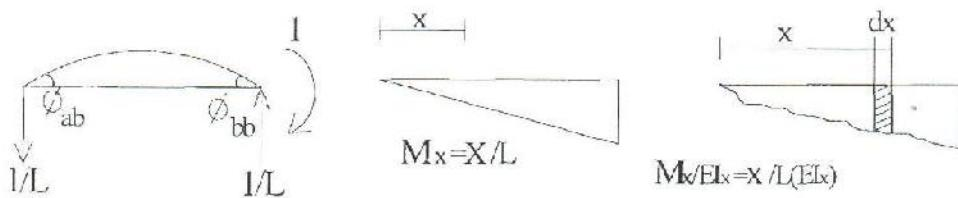
$$\Phi_{ab} = (b-a) \int_0^L \frac{M}{EI} dx = \frac{1}{L} \int_0^L \left( \frac{x}{L} \right) \frac{dx}{EI_C n_x} (L-x)$$
