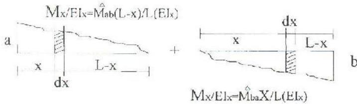
$$I) \Delta = - \int_0^L \left( \frac{M_{ab}^\Delta}{EI_C n_x} \frac{L-x}{L} dx \right) (L-x) - \int_0^L \left( \frac{M_{ba}^\Delta}{EI_C n_x} \frac{x}{L} dx \right) (L-x) = - \frac{M_{ab}^\Delta L^2}{EI_C} C_1 + \frac{M_{ba}^\Delta L^2}{EI_C} C_2$$
