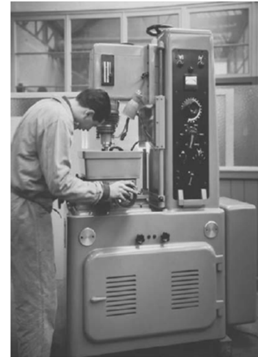
FIGURE 1.6 First industrial EDM machine in the world. Presentation of the Eleroda DI at the EMO exhibition in Milan Italy, 1955. (Courtesy of Charmilles, 560 Bond St., Lincolnshire, IL.)
