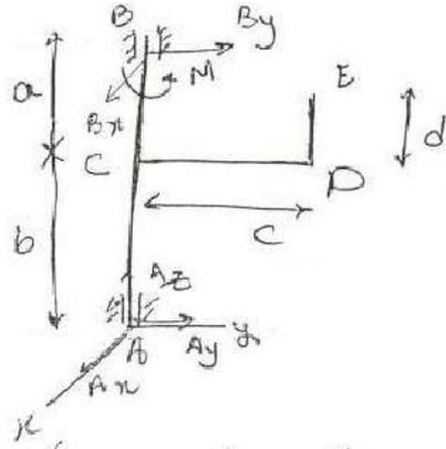
$$\begin{aligned} \gamma &= 5 \text{ lb/ft} & M &= 20 \text{ lb-ft} \\ a &= 4 \text{ ft} & y &= 32.2 \\ b &= 2 \text{ ft} & \omega &= 10 \text{ rad/s} \\ c &= 2 \text{ ft} \\ d &= 2 \text{ ft} \end{aligned}$$
