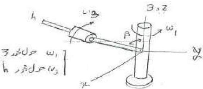
$$\begin{aligned}\vec{\omega} &= \vec{\omega}_1 + \vec{\omega}_2 + \vec{\omega}_3 \\ &= \omega_1 \hat{k} + \beta \hat{i} + \omega_3 \hat{h} \\ &= \omega_1 \hat{k} + \beta \hat{i} + \omega_3 (\cos\beta \hat{k} - \sin\beta \hat{j})\end{aligned}$$
