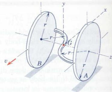
**Solution.** The motion is identified as parallel-plane motion since the planes of motion of all parts of the system are parallel. The free-body diagram shows the normal forces and friction forces at  $A$  and  $B$  and the total weight  $mg$  acting through the mass center  $G$ , which we take as the origin of coordinates that rotate with the body.
