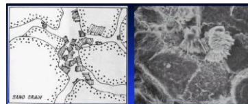
Classical Kaolinite "booklets" - potential for formation damage From Nissham 1977, SPE 6959
