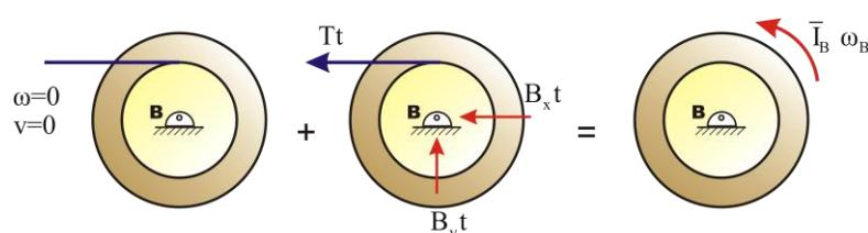
$$\sum M_B : 0 + Tt(r_i) = \bar{I} \omega_B \Rightarrow T(3)(0.1) = 0.25(\frac{1.5V_c}{0.1}) \quad (2) \quad (1),(2) \Rightarrow V_c = 3.23 \text{ (m/s)} \downarrow$$
