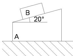
$$\vec{a}_B = \vec{a}_A + \vec{a}_{B/A} , \quad \vec{a}_B = \sqrt{120^2 + 80^2 - 2(120)(80) \cos 20^\circ}$$
