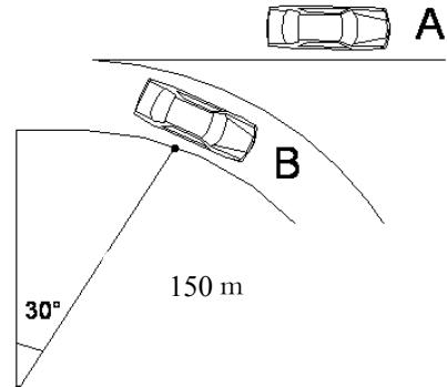
$$20.8 \frac{\text{m}}{\text{s}} = v_A = \left[ 75 \frac{\text{km}}{\text{h}} \rightarrow \right] \quad a_A = 1.5 \frac{\text{m}}{\text{s}^2} \quad \vec{v}_{A/B} = ?$$
