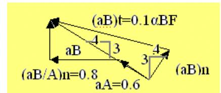
$$\begin{cases} (\vec{a}_B)_n + (\vec{a}_B)_t = \vec{a}_A + (\vec{a}_{B/A})_n + (\vec{a}_{B/A})_t \\ (a_B)_n = 0.625 \text{ m/s}^2, (a_B)_t = 0.1 a_{BF} \Rightarrow [0.625 \rightarrow] + [0.1 a_{BF} \leftarrow] = [0.625 \rightarrow] + [0.8 \leftarrow] + [0.2 \alpha \uparrow] \\ (\vec{a}_{B/A})_n = 0.2\omega^2 = 0.8 \text{ m/s}^2, (\vec{a}_{B/A})_t = 0.2\alpha \\ \Rightarrow \alpha = 12(\text{rad/s}) \end{cases}$$
