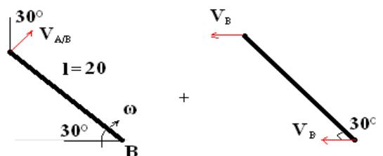
$$\vec{V}_{A/B} = \vec{V}_A \quad \Rightarrow \vec{V}_A = \vec{V}_B = 25 \text{ (Cm/s)}$$
