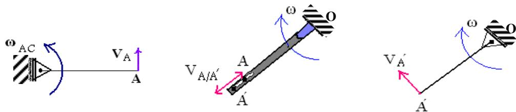
$$V_{A'} = 0.225\sqrt{2} \quad \omega = 0.45\sqrt{2} \text{ m/s } 45^\circ$$
