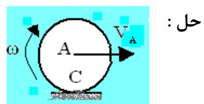
$$V_A = \text{ثابت} \Rightarrow \omega = \text{ثابت} \Rightarrow \alpha = 0$$
