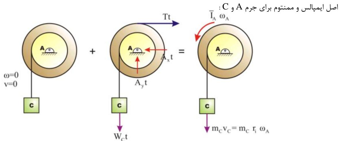
$$\sum M_A : 0 + W_C t(r_i) - Tt(r_o) = m_c v_c r_i + \bar{I} \omega_A \Rightarrow 10g(3)(0.1) - T(3)(0.15) = 10V_c (0.1) + 0.25(\frac{V_c}{0.1}) \quad (1)$$
