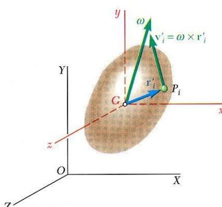
$$\vec{w} \times \vec{r}_i' = \begin{vmatrix} \vec{i} & \vec{j} & \vec{k} \\ w_x & w_y & w_z \\ x_i & y_i & z_i \end{vmatrix} = (w_y z_i - w_z y_i) \vec{i} + (w_z x_i - z_i w_x) \vec{j} + (w_x y_i - w_y x_i) \vec{k}$$
