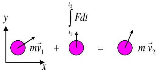
$$\begin{cases} mv_{2_x} = \int_{t_1}^{t_2} F_x dt + mv_{1_x} \\ mv_{2_y} = \int_{t_1}^{t_2} F_y dt + mv_{1_y} \end{cases} \quad \begin{array}{l} \rightarrow \\ \uparrow \end{array}$$
