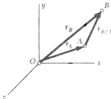
$$\frac{d}{dt}(\vec{r}_{B/A}) = \frac{d}{dt}(\vec{r}_B) - \frac{d}{dt}(\vec{r}_A) \Rightarrow \vec{v}_{B/A} = \vec{v}_B - \vec{v}_A \quad : A$$
