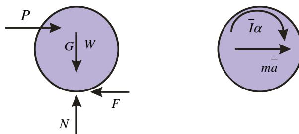
$$\begin{aligned} \bar{a} &= r\alpha & \Sigma M_c &= (\Sigma M_c)_{eff} \\ \Sigma M_c &= (\Sigma M_c)_{eff} \Rightarrow P \times r = \bar{I}\alpha + m\bar{a}r \\ \Rightarrow 40(0.5) &= (\frac{1}{2}(\frac{50}{32.2})(0.5)^2 + \frac{50}{32.2}(0.5)^2)\alpha \Rightarrow \alpha = 34.35 \text{ (rad/s}^2\text{)} \end{aligned}$$
