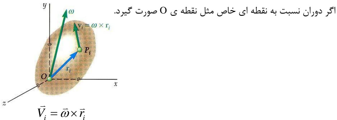
$$\begin{aligned} T &= \frac{1}{2} \sum_{i=1}^n (\Delta m_i) v_i^2 = \frac{1}{2} \sum_{i=1}^n (\vec{\omega} \times \vec{r}_i)^2 \Delta m_i \\ &= \frac{1}{2} (I_x w_x^2 + I_y w_y^2 + I_z w_z^2 - 2I_{xy} w_x w_y - 2I_{yz} w_y w_z - 2I_{zx} w_z w_x) \end{aligned}$$
