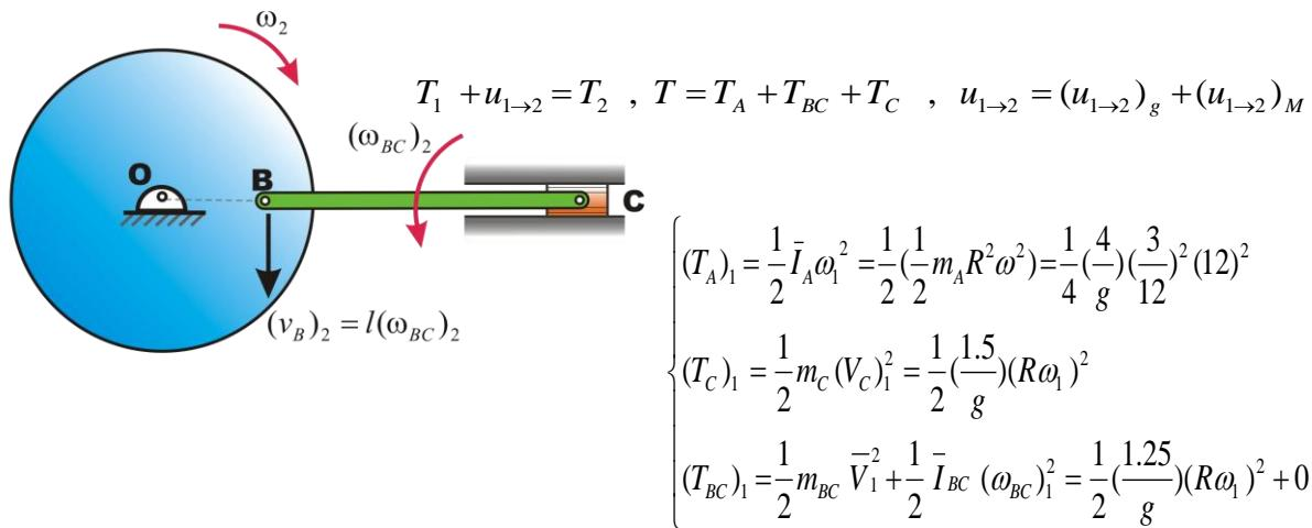
$$\left\{ \begin{array}{l} (T_A)_1 = \frac{1}{2} \bar{I}_A \omega_1^2 = \frac{1}{2} \left( \frac{1}{2} m_A R^2 \omega_1^2 \right) = \frac{1}{4} \left( \frac{4}{g} \right) \left( \frac{3}{12} \right)^2 (12)^2 \\ (T_C)_1 = \frac{1}{2} m_C (V_C)_1^2 = \frac{1}{2} \left( \frac{1.5}{g} \right) (R\omega_1)^2 \\ (T_{BC})_1 = \frac{1}{2} m_{BC} \bar{V}_1^2 + \frac{1}{2} \bar{I}_{BC} (\omega_{BC})_1^2 = \frac{1}{2} \left( \frac{1.25}{g} \right) (R\omega_1)^2 + 0 \end{array} \right.$$
