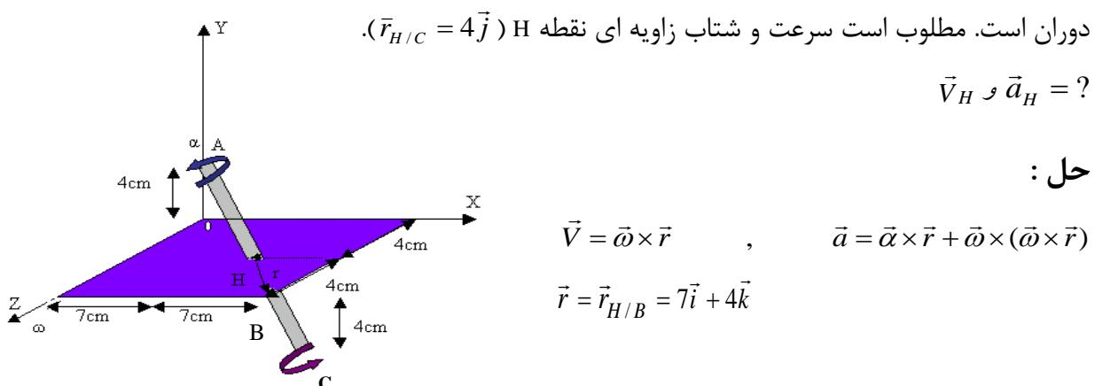
$$\vec{V} = \vec{\omega} \times \vec{r}, \quad \vec{a} = \vec{\alpha} \times \vec{r} + \vec{\omega} \times (\vec{\omega} \times \vec{r})$$
