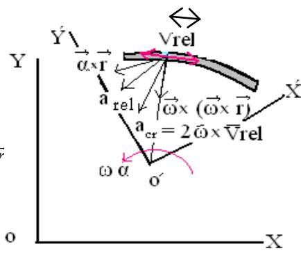
$$\vec{a}_p = \ddot{\vec{S}} = \frac{d}{dt}(\vec{R} + \vec{r}' + \vec{\omega} \times \vec{r}) = \ddot{\vec{R}} + \frac{d}{dt}(\vec{r}') + \frac{d}{dt}(\vec{\omega} \times \vec{r}) = \ddot{\vec{R}} + (\vec{r}' + \vec{\omega} \times \vec{r}') + \frac{d}{dt}(\vec{\omega}) \times \vec{r} + \vec{\omega} \times \frac{d\vec{r}}{dt}$$
