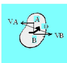
$$\begin{aligned} V_A &\parallel V_B \\ V_A &\perp AB \end{aligned}$$
