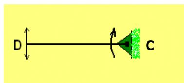
$$\Rightarrow V_D = 0.225 \omega_{DC} = 0.45 \text{ m/s} \Rightarrow \omega_{DC} = 2 \text{ rad/s}$$
