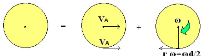
$$\Rightarrow V_{C/A} = V_A = r\omega \Rightarrow 13.9 = r\omega \Rightarrow \omega = \frac{13.9}{0.61/2}$$
