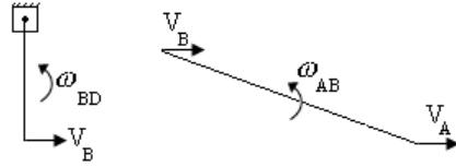
$$\begin{cases} \vec{V}_B = \vec{V}_A + \vec{V}_{B/A} \Rightarrow [V_B \rightarrow] = [V_A \rightarrow] + [3\omega_{AB} \downarrow 30^\circ] \Rightarrow \omega_{AB} = 0 , V_B = V_A = 2.5 \text{ m/s} \\ V_B = \omega_{BD} (1.25) \\ \Rightarrow \omega_{BD} = 2.5 / 1.25 = 2 \text{ rad/s} \end{cases}$$
