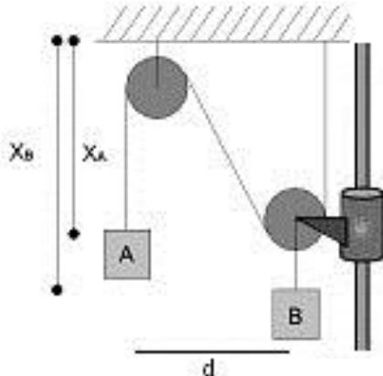
$$L = \text{ثابت} \quad L = x_A + \sqrt{d^2 + x_B^2} + x_B$$
