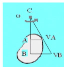
$$\begin{aligned} V_A &\parallel V_B \\ V_A &\perp AB \\ V_A &\neq V_B \end{aligned}$$
