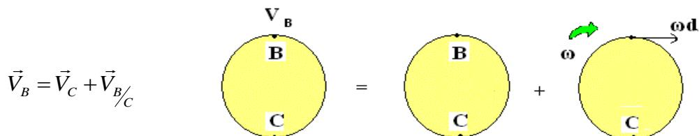
$$\Rightarrow \vec{V}_B = 0 + [d\omega \rightarrow] = [2 \times 13.9 \rightarrow] = [27.8 \text{ m/s} \rightarrow]$$
