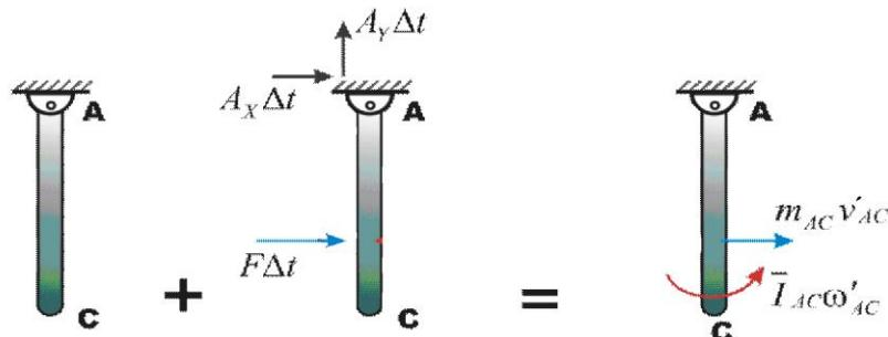
$$\sum M_A: 0 + F.t(1.5) = \bar{I}_{AC} \omega'_{AC} + m_{AC} \bar{V}'_{AC} (1.5) \Rightarrow F = 453.42 \text{ (lb)}$$
