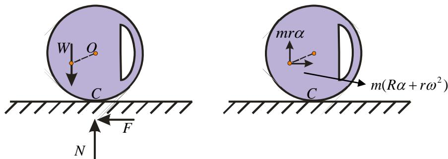
$$\Sigma M_C = (\Sigma M_C)_{\text{eff}} \Rightarrow W \times r = -\bar{I}\alpha - mr\alpha r - m(R\alpha + r\omega^2)R$$
