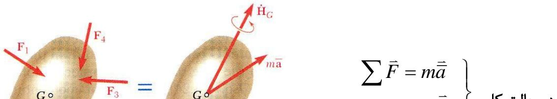
$$\left. \begin{array}{l} \sum \vec{F} = m \bar{\vec{a}} \\ \sum m_G = \vec{H}_G = \bar{I} \vec{d} \end{array} \right\}$$
