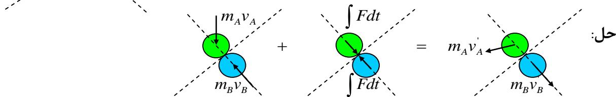
$$(v_A')_t = (v_A)_t = 8\sin(40^\circ) = 5.15 \frac{\text{m}}{\text{s}} , \quad (v_B')_t = (v_B)_t = 0$$
