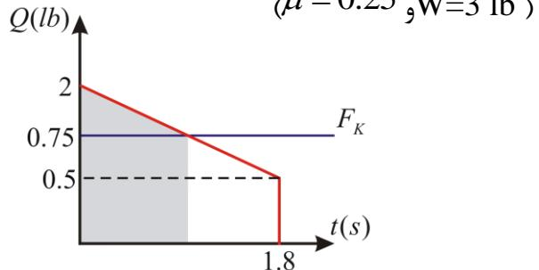
$$\vec{L}_2 = \vec{I}_{mp_{1 \rightarrow 2}} + \vec{L}_1 \quad , \quad \vec{L}_1 = mv_1 = 0 \quad , \quad I_{mp} = \int_0^t Q dt - \int_0^t F_k dt$$
