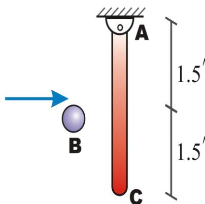
$$W_B = 2 \text{ (lb)} \quad \text{و} \quad W_{AC} = 10 \text{ (lb)} \quad , \quad e = 0.4$$
