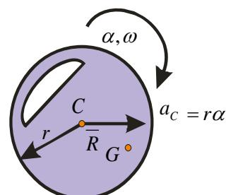
$$\begin{aligned} \vec{a}_G &= \vec{a}_C + \vec{a}_{G/C} \quad , \quad a_c = r\alpha \\ \vec{a}_G &= (r\alpha \rightarrow) + (\bar{R}\alpha \swarrow) + (\bar{R}w^2 \nwarrow) \end{aligned}$$
