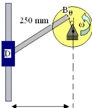
$$\omega = 500 \text{ rpm} = \frac{500 \times 2\pi}{60} = 52.36 \text{ rad/s} \quad \text{حل :}$$
