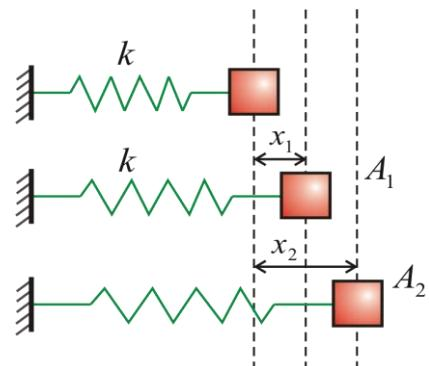
$$\left. \begin{array}{l} T_1 + U_{1 \rightarrow 2} = T_2 \\ T_1 + V_1 - V_2 = T \end{array} \right\} \Rightarrow T_1 + V_1 = T_2 + V_2$$
