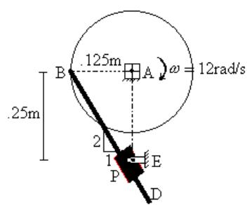
$$\begin{cases} \vec{V}_B = .125 \times 12 = 1.5 m/s \uparrow \\ V_B = \omega_{BD}(r_{B/C}) = \omega_{BD}(0.125 + 0.5) \Rightarrow \omega_{BD} = 2.4 rad/s \\ \Rightarrow V_p = \omega_{BD}(r_{P/C}) = 2.4(0.56) = 1.34 m/s \end{cases}$$
