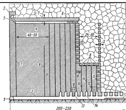
1-2—intermediate crosscut; 2—haulage entry; 4—ventilating entry; 3—inclined thin cut; 6—level pillar; 7, 8—boreholes; 8—4-section shield; 10, 11, 12, 13—coal chute pocket; 16—service raise; 16—breakthrough; 17—ventilating through-cut; 18—break!
