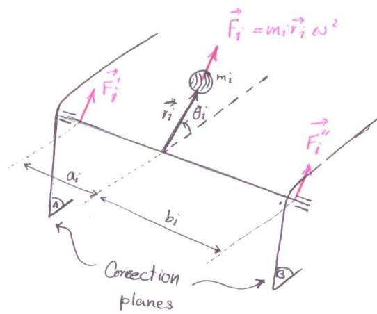
$$\begin{cases} \vec{F}_i^a = \left( \frac{b_i}{a_i + b_i} m_i \right) \vec{r}_i \omega^2 \\ \vec{F}_i^b = \left( \frac{a_i}{a_i + b_i} m_i \right) \vec{r}_i \omega^2 \end{cases}$$
