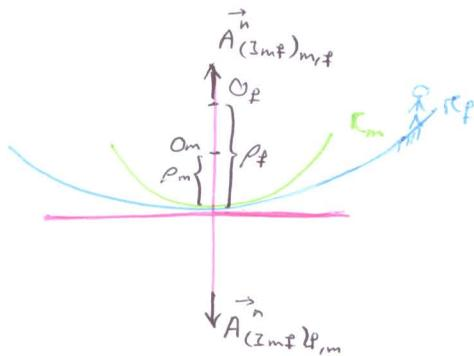
$$\vec{A}_{(Imf)_{m,f}}^n = \frac{r_f r_m}{r_f - r_m} (\omega_m - \omega_f)^2 \vec{j}$$
