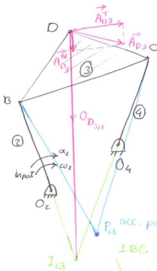
$$\left[ \left( \vec{A}_{C_3}^n \right) + \left( \vec{A}_{C_3}^t \right) \right] = \left( \vec{A}_{B_3}^n + \vec{A}_{B_3}^t \right) + \left( \vec{A}_{C_3/B_3}^n + \vec{A}_{C_3/B_3}^t \right) \quad (*)$$
