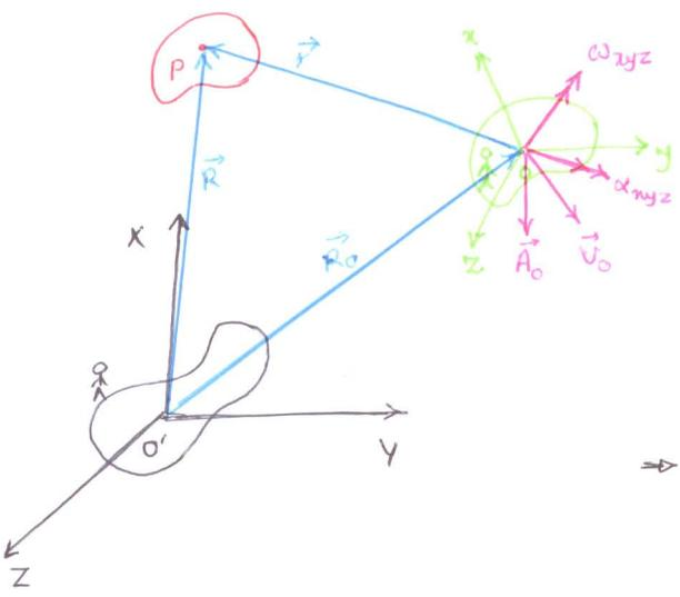
$$\begin{aligned} \vec{R} &= \vec{r} + \vec{R}_0 \\ \vec{V}_{xyz} &= \vec{V}_{xyz} + \vec{V}_0 + \vec{\omega} \times \vec{r} \\ \vec{A}_{xyz} &= (\vec{A}_{xyz} + \vec{\omega} \times \vec{V}_{xyz}) + \vec{A}_0 + \vec{\alpha} \times \vec{r} + \vec{\omega} \times \left[ \left( \frac{d\vec{r}}{dt} \right)_{xyz} + \vec{\omega} \times \vec{r} \right] \end{aligned}$$
