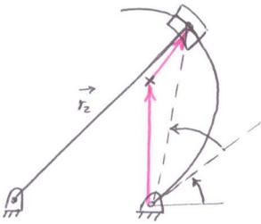
$$\vec{r}_k = i r_k \dot{\theta}_k e^{i\theta_k} = r_k \omega_k (i \cos \theta_k - \sin \theta_k), \quad \vec{r} = \vec{0}$$
