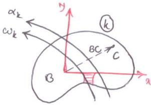
$$\vec{A}_{Ck} = \vec{A}_{Bk} + \vec{\alpha}_k \times \vec{BC} + \vec{\omega}_k \times (\vec{\omega}_k \times \vec{BC})$$
