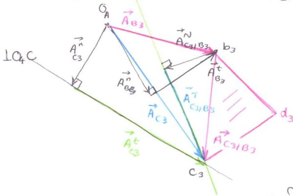
$$\alpha_3 = \frac{|\vec{A}_{C_3/B_3}^t|}{(BC)} \quad \text{C.W}$$
