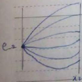
$$\frac{\partial F}{\partial y} - \frac{d}{dx} \left( \frac{\partial F}{\partial y'} \right) = 0$$
