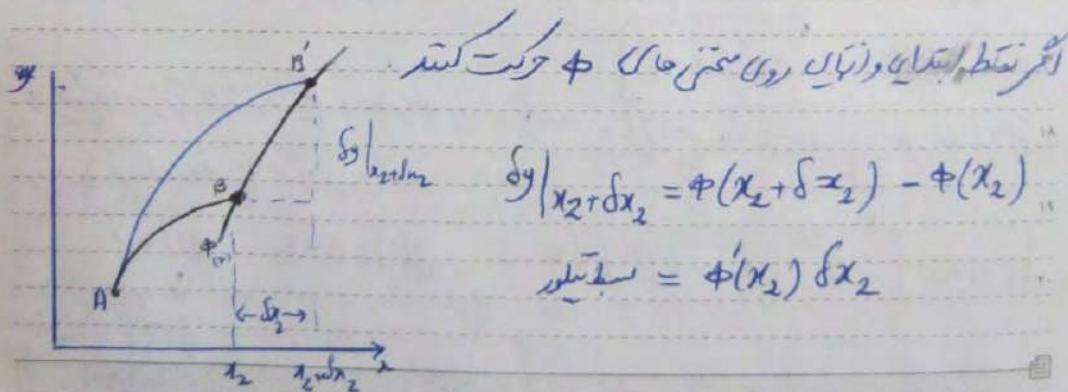
$$\delta I = \left( F - y' \frac{\partial F}{\partial y'} \Big|_{x_2}^{\bar{x}_2} \right) \delta x_2 + \frac{\partial F}{\partial y'} \left( \phi'(x_2) \delta x_2 \right)$$
