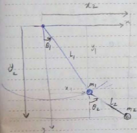
$$T = \frac{1}{2} m_1 v_1^2 + \frac{1}{2} m_2 v_2^2$$
