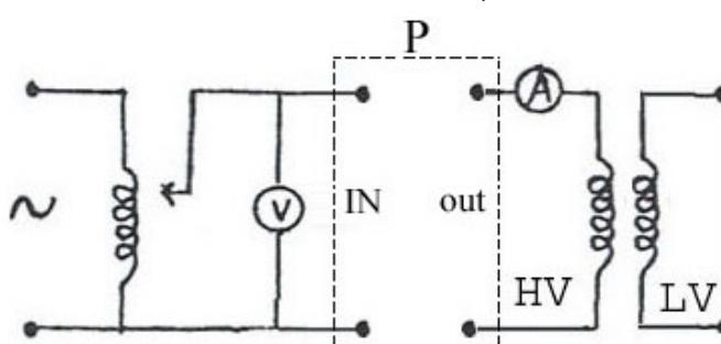
$$P_{cu} = I^2 R_{eq} \rightarrow R_{eq} = P / I_{SC}^2$$
