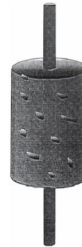
Figure 42 Sketch of a tension specimen ready for testing.
