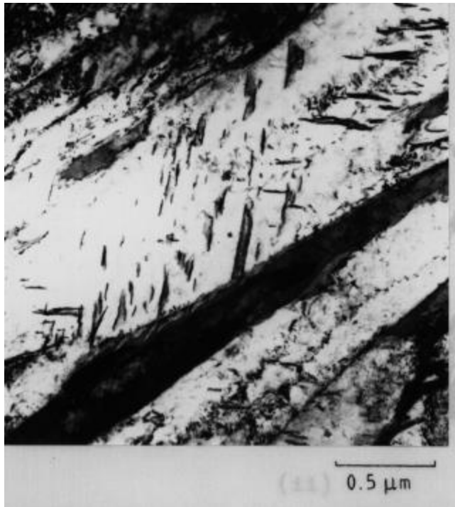
The microstructure of lower bainite
