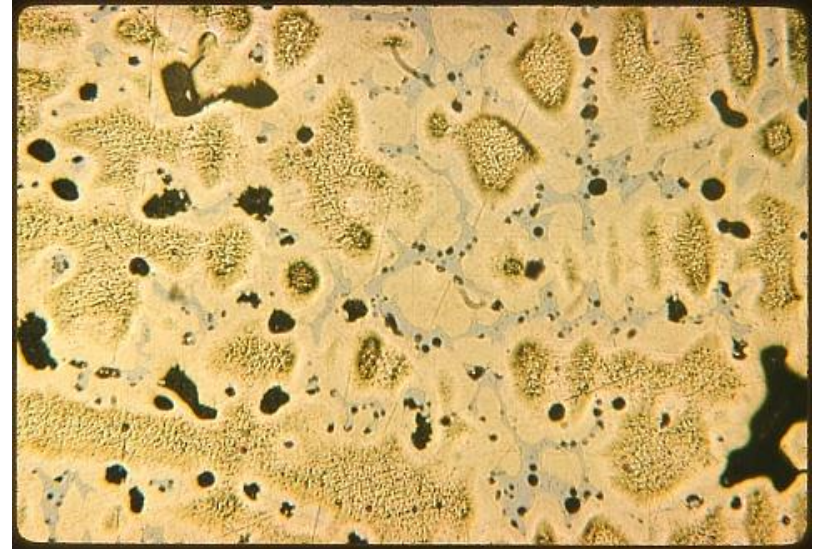
At 200X the bluish-white delta microconstituent can be seen. The black areas in these two photomicrographs are either shrinkage cavities or lead particles
