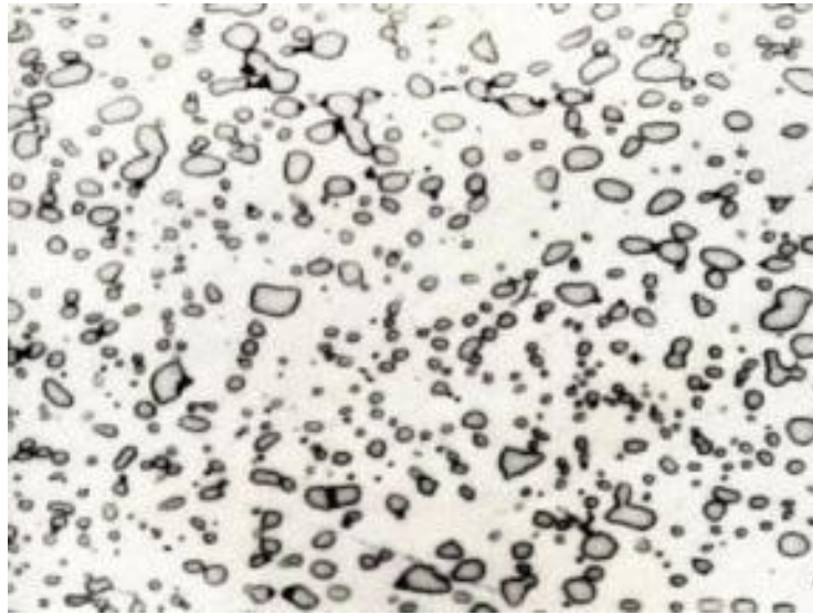
Spheroidized cementite in a ferrite matrix
