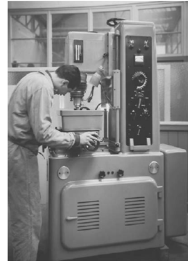
FIGURE 1.6 First industrial EDM machine in the world. Presentation of the Eleroda DI at the EMO exhibition in Milan Italy, 1955. (Courtesy of Charmilles, 560 Bond St., Lincolnshire, IL.)
