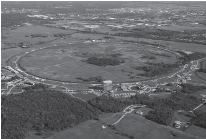
FIGURE 14.1 An aerial view of the Tevatron at the Fermi National Accelerator Laboratory. Beams of protons and antiprotons circulate in opposite directions around the 1-km ring and collide at two locations, at the upper center and lower left. (Courtesy Fermi National Accelerator Laboratory.)
