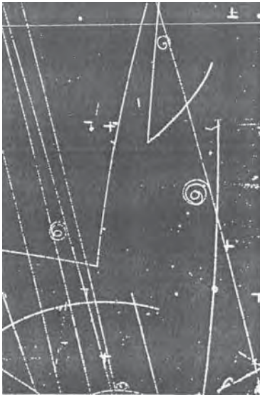
FIGURE 14.3 A bubble chamber photograph of a reaction between particles. At right is shown a diagram indicating the particles that participate in the reaction. An incident pion collides with a proton in the liquid hydrogen, producing a K^0 and a \Lambda^0 , both of which subsequently decay. (Photo Courtesy Lawrence Berkeley National Laboratory.)
