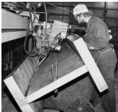
FIG. 5-17 Welding three large steel plates into a single solid section (Courtesy of The Lincoln Electric Company)
