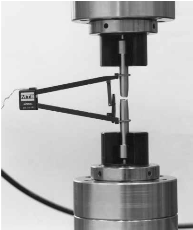
FIG. 1-8 Typical tensile-test specimen with extensometer attached; the specimen has just fractured in tension. (Courtesy of MTS Systems Corporation)
