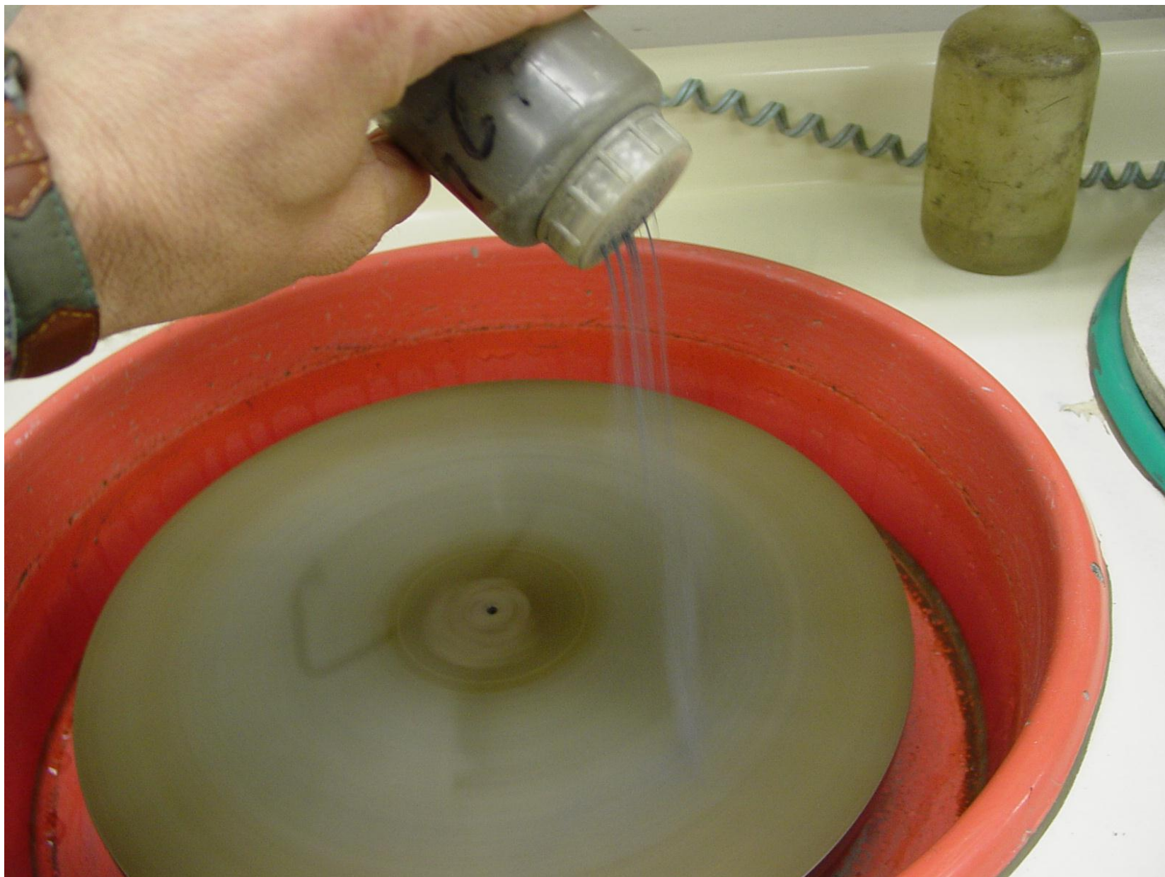
Putting 240-grit abrasive on spinning, wet wheel.
