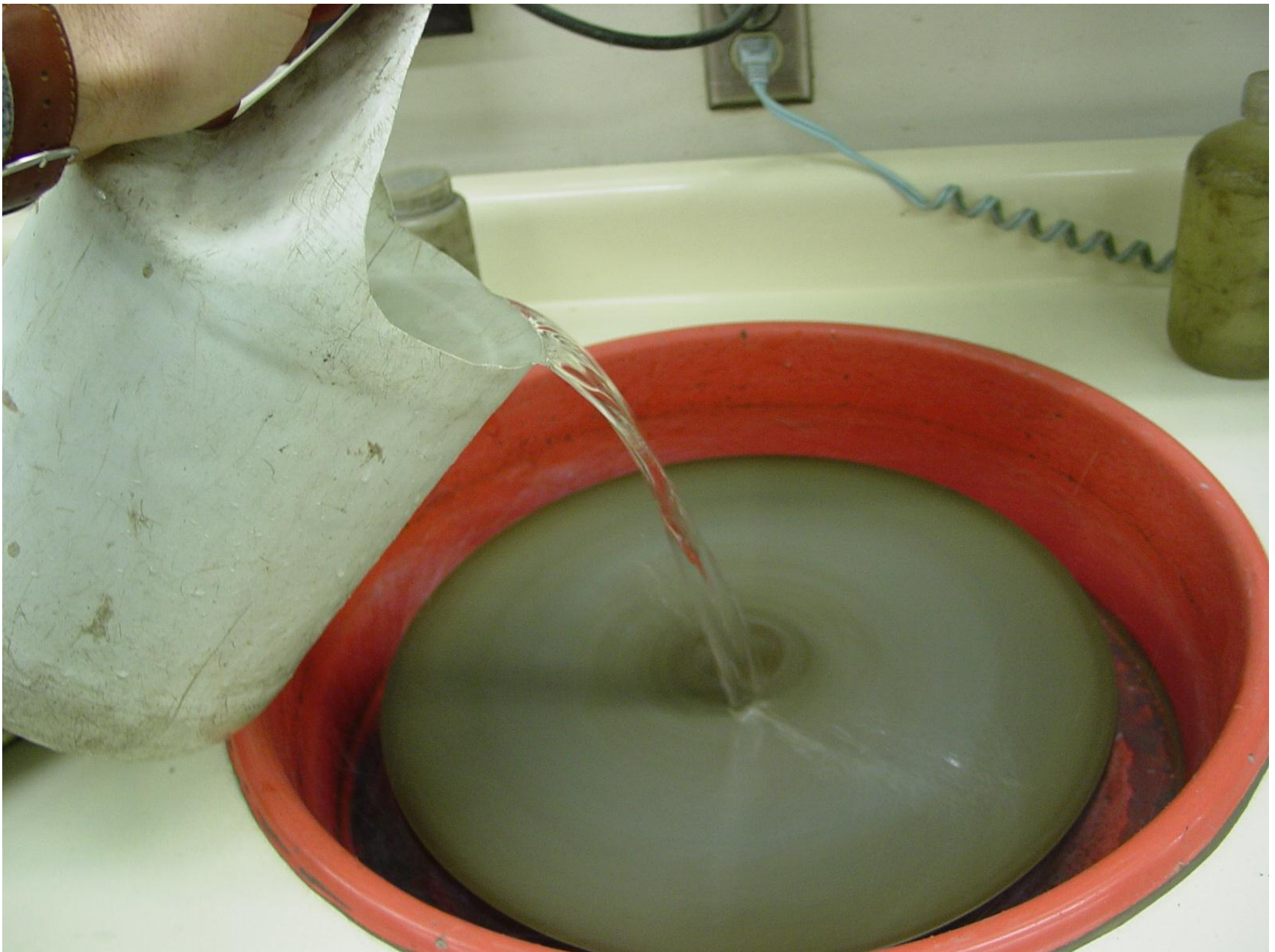
Pouring water on the grinding wheel for initial cleaning.
