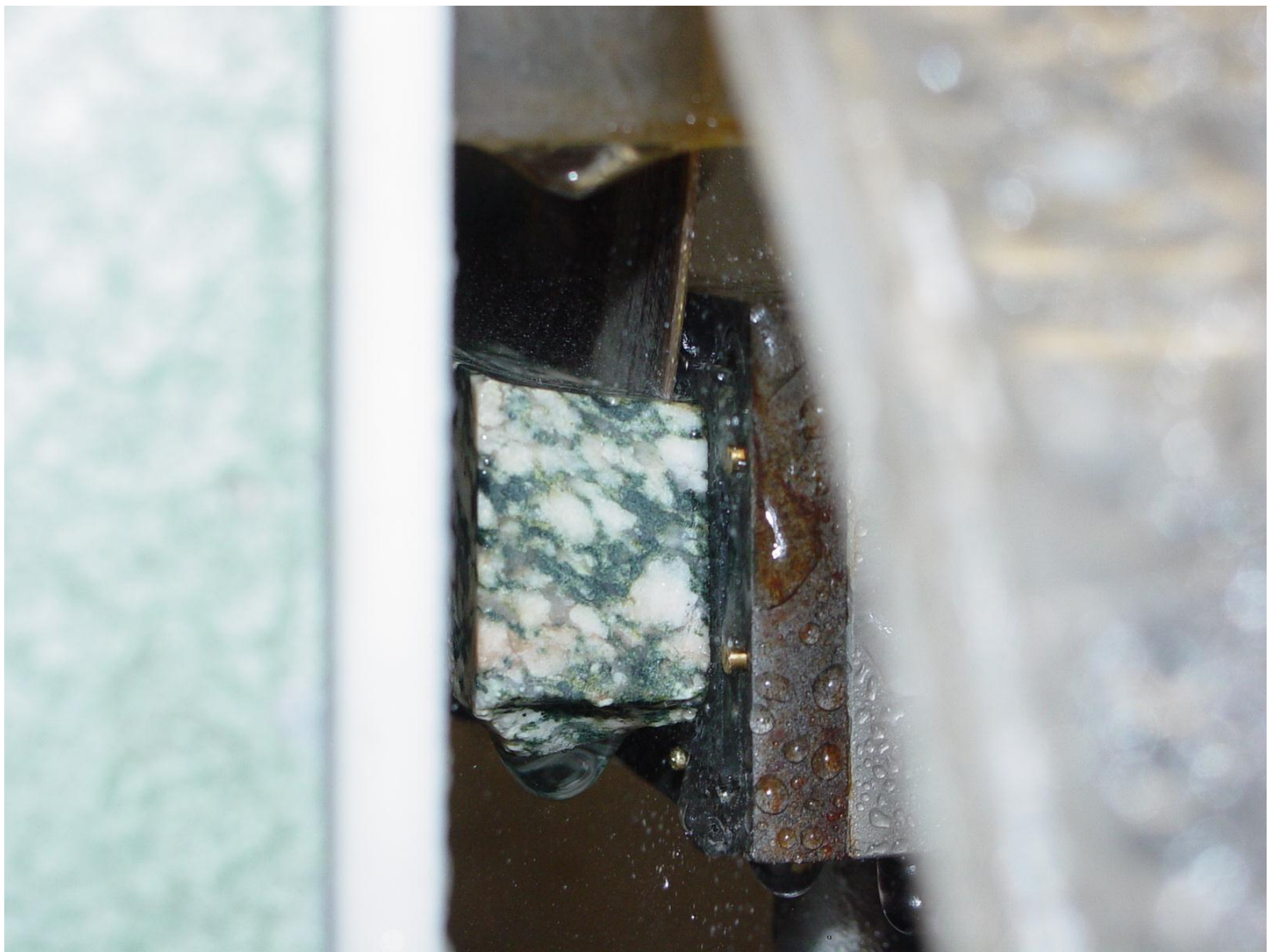
Chip nearly cut from slide.
