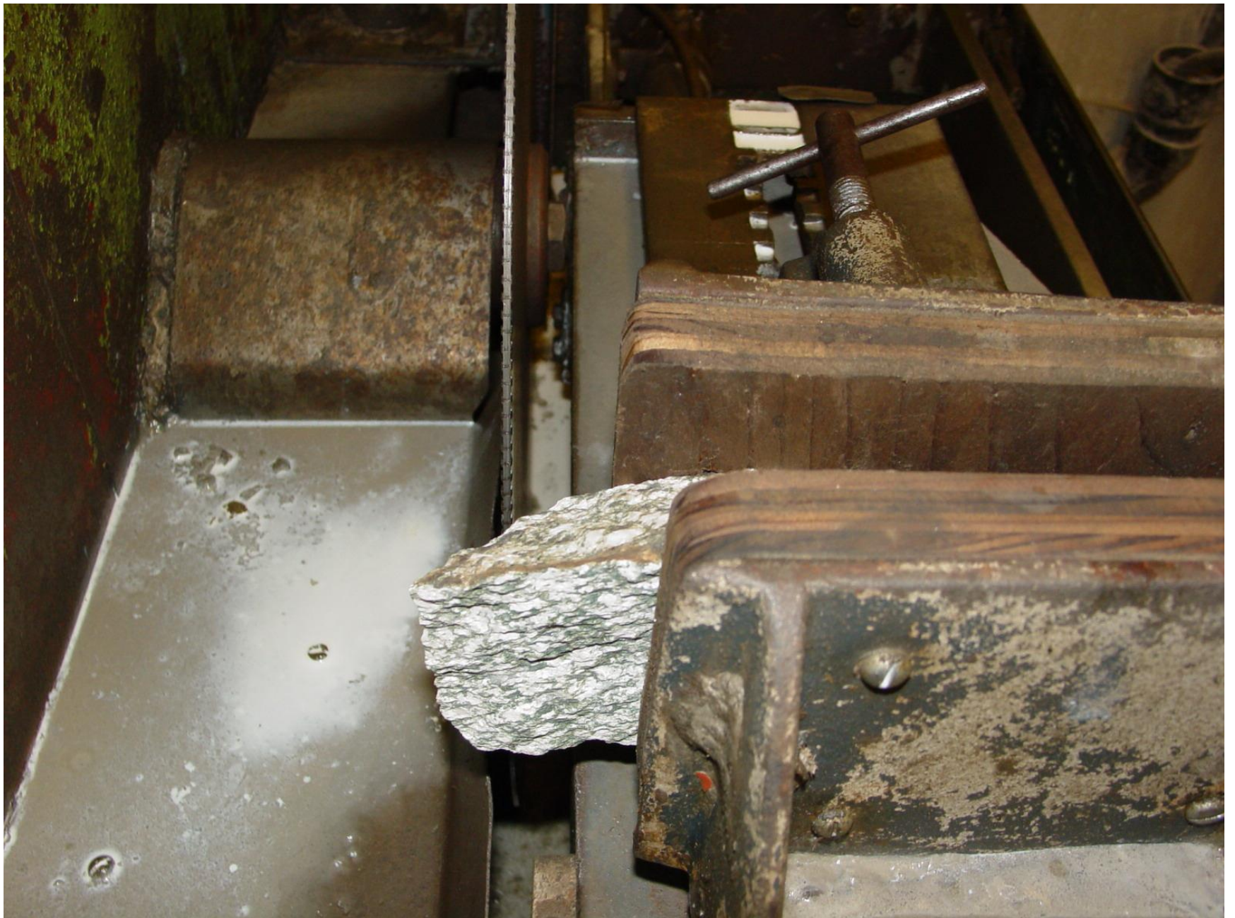
Rock ready for first cut. Note that it sticks out extra far to allow for second cut without removing from clamp.
