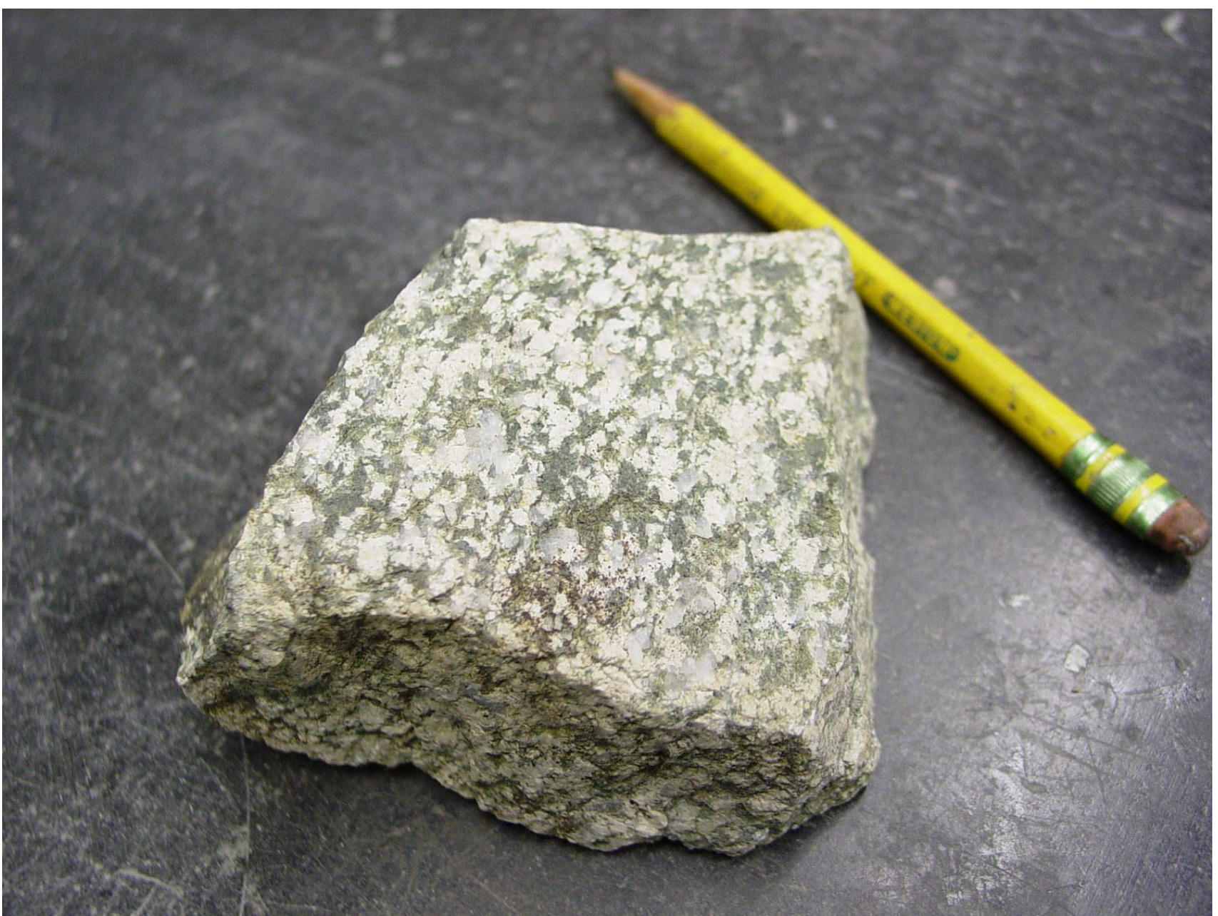
Rock prior to cutting. Pencil for scale. Note that this rock was not marked before cutting, but normally it would be.
