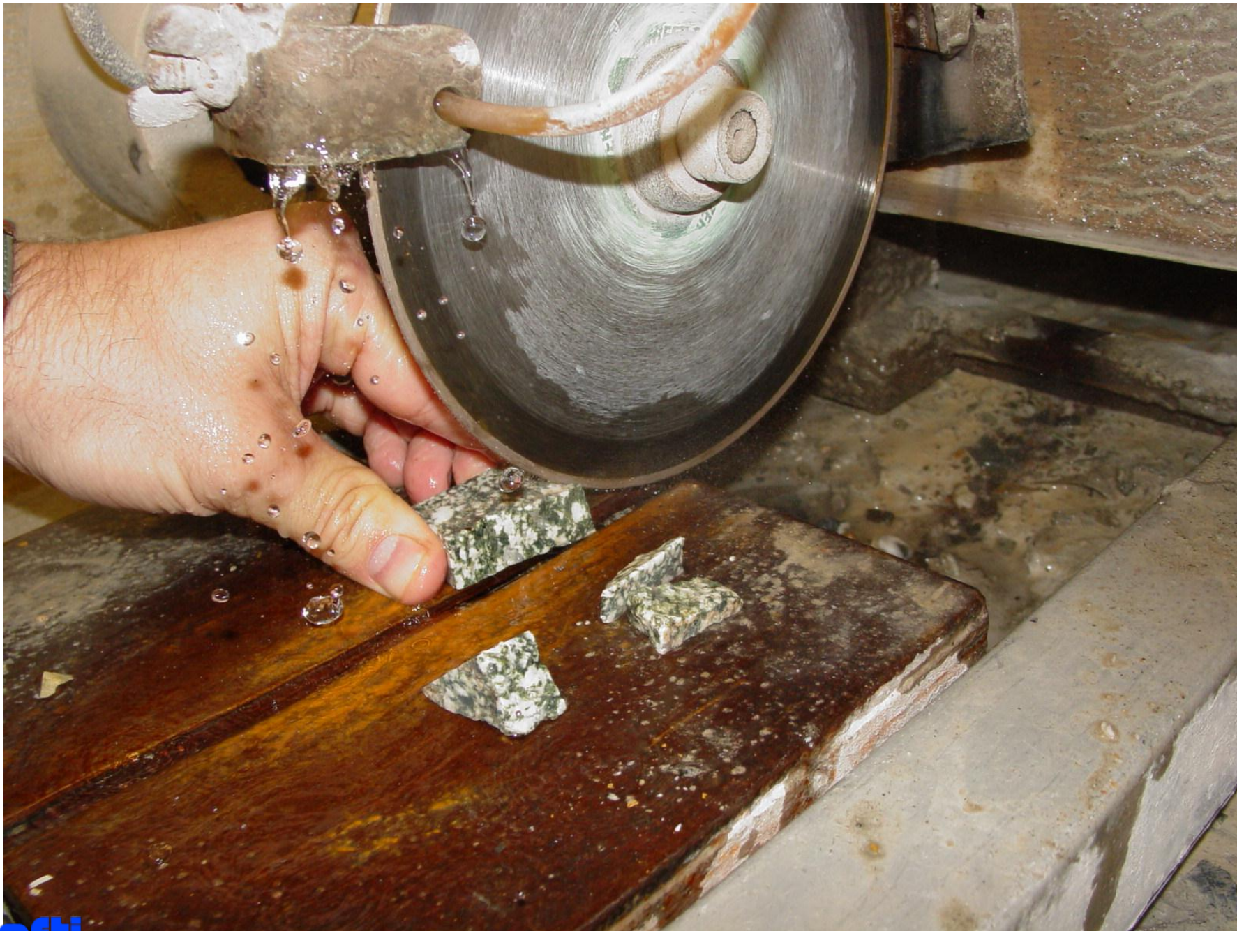
Final cut for the chip.
