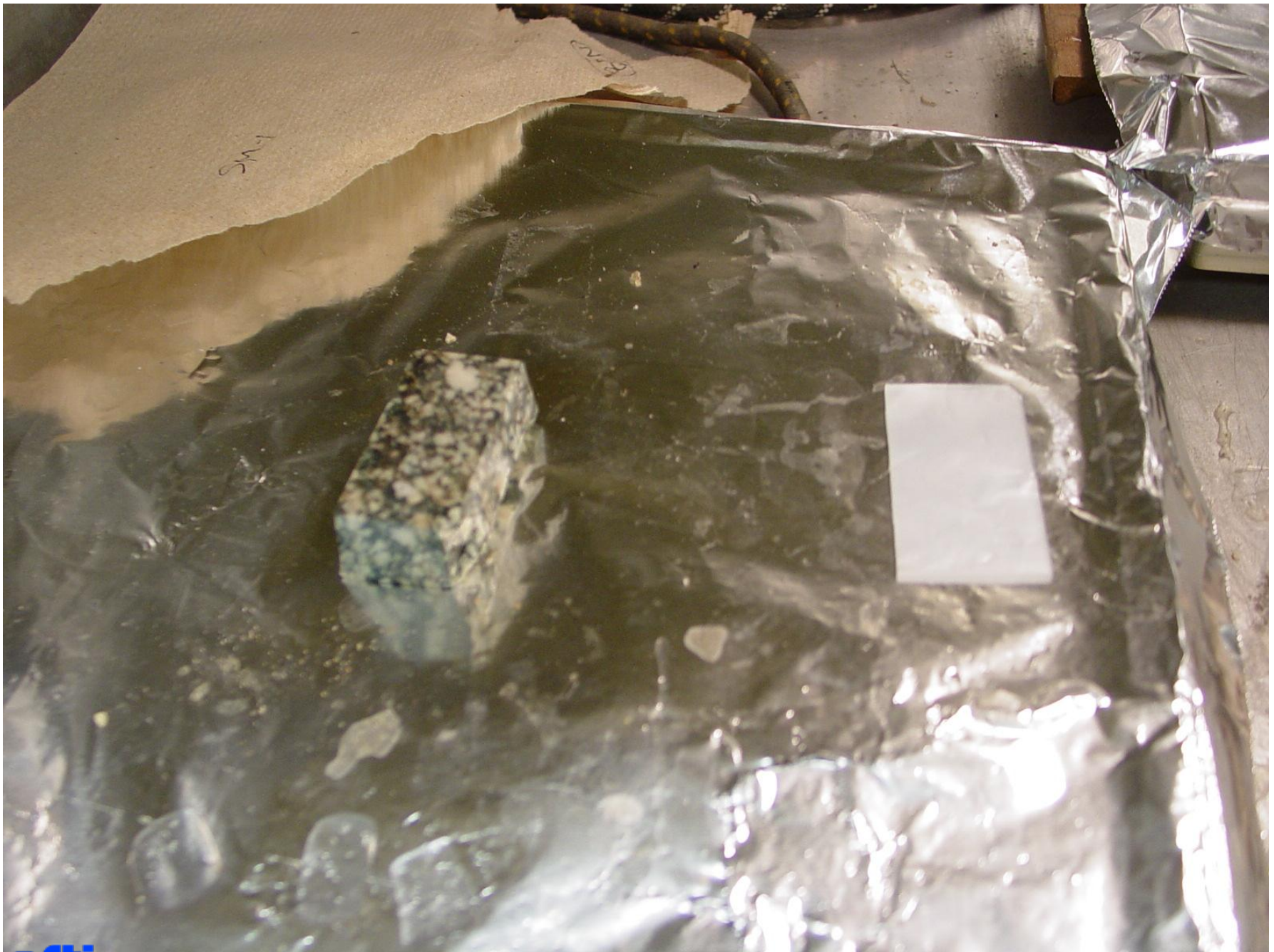
Cut and polished chip warming up on the hot plate.
