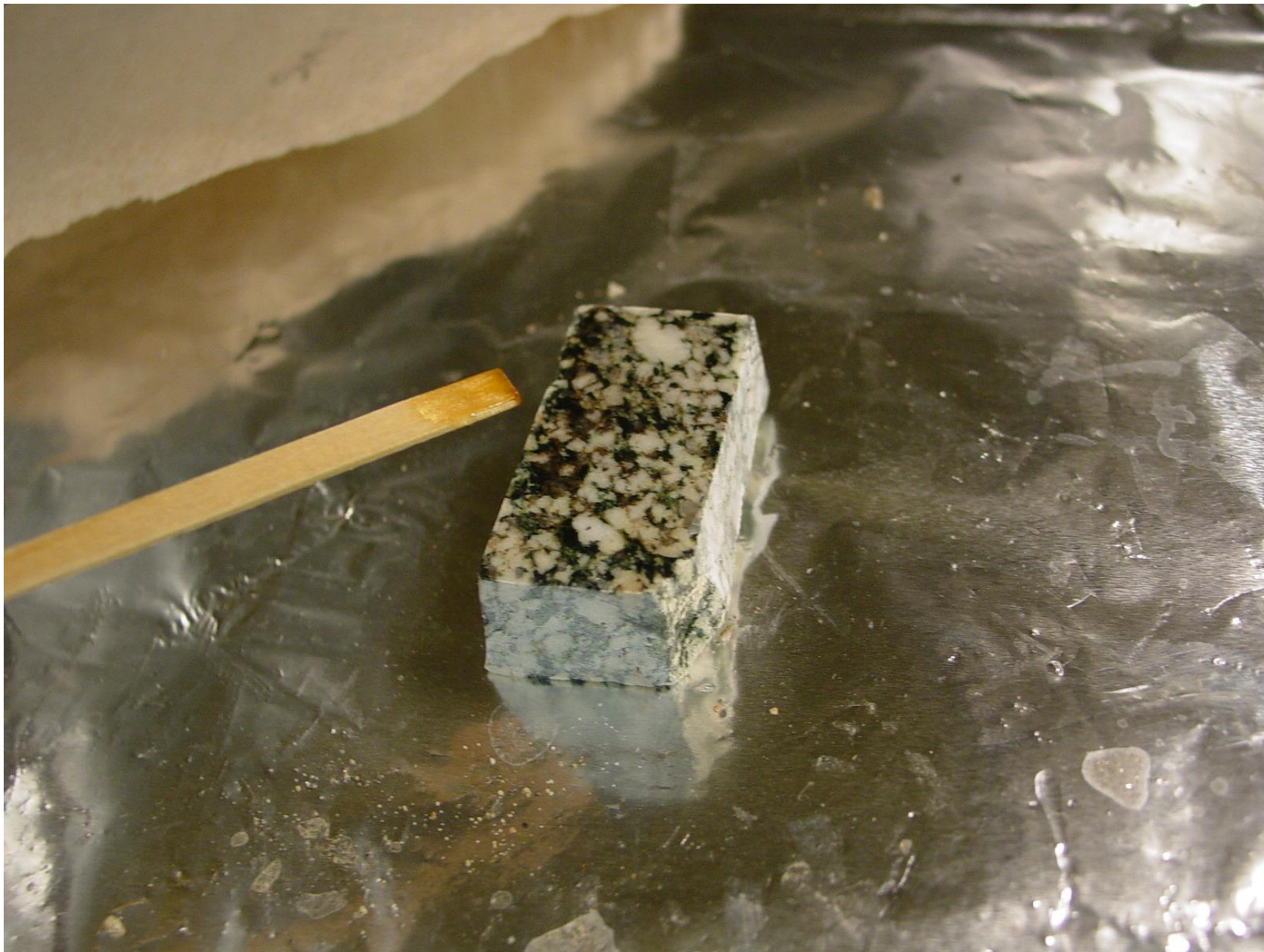
Chip coated with epoxy after allowing it to penetrate.
