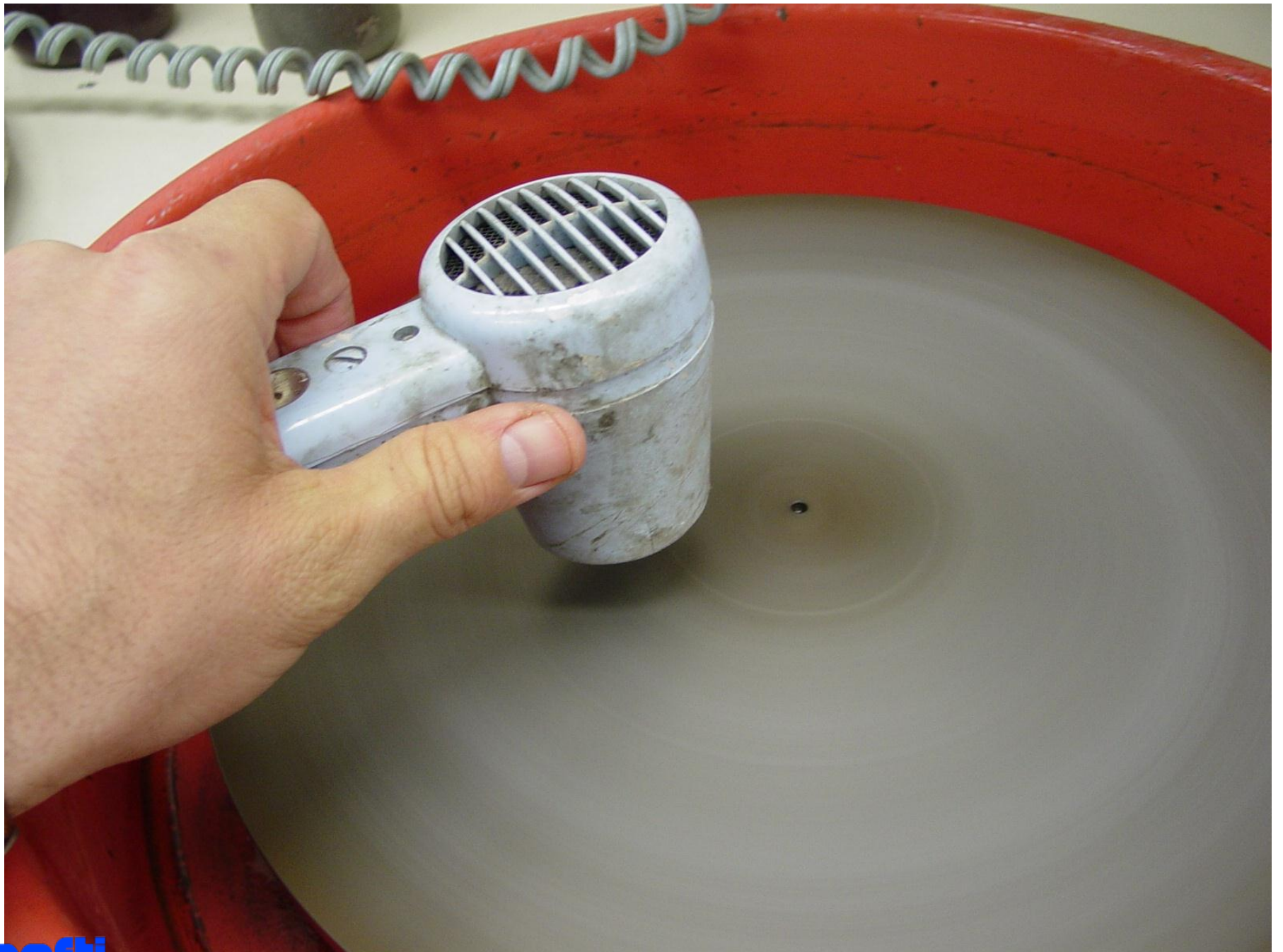
Final drying of wheel with hair dryer.
