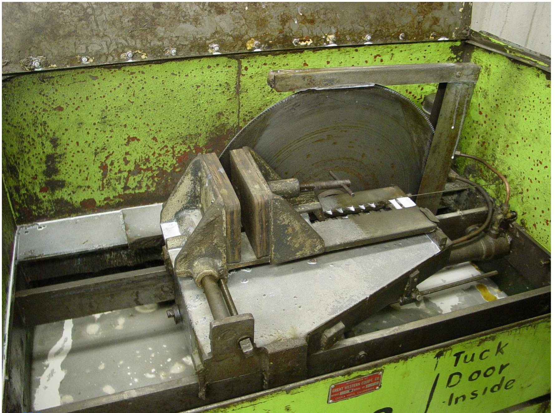
Slab saw. Note location for crank in bottom center.
