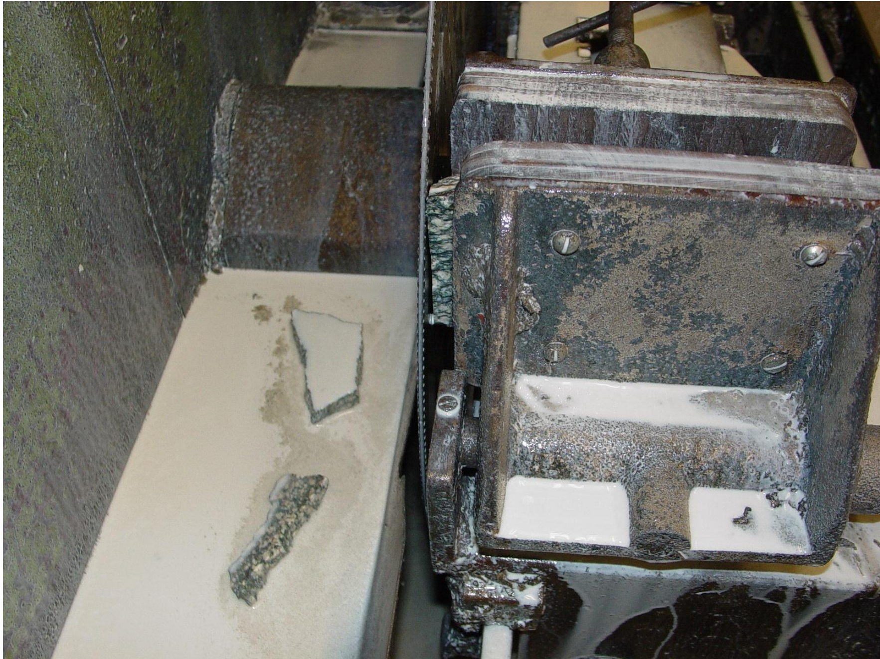
nafti.ir After second cut: slab complete (piece lying on catch tray at left).
