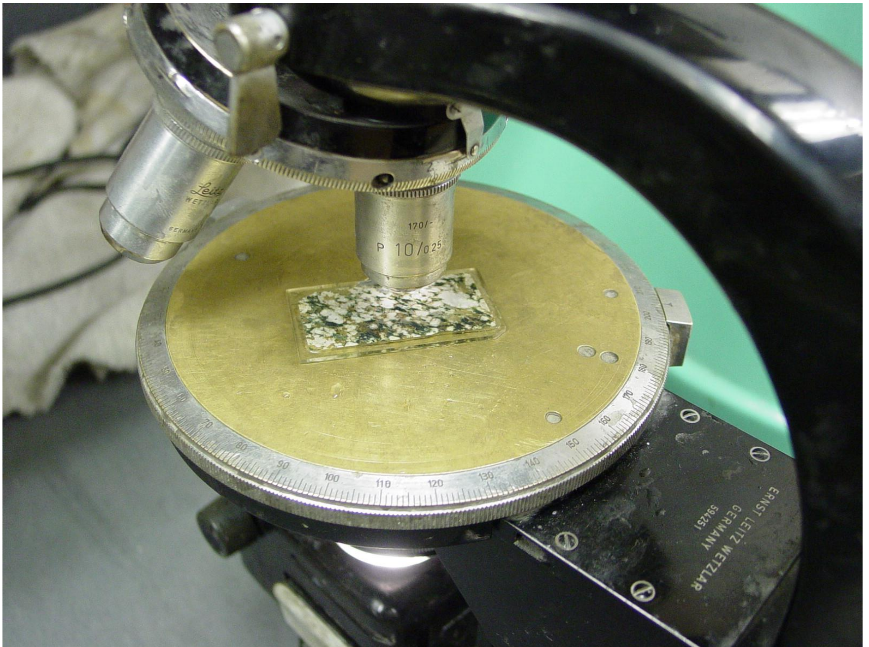
Checking the slide thickness using the microscope.
