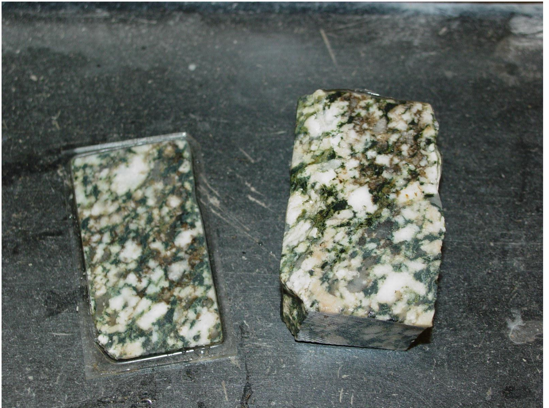
Chip and slide separated.
