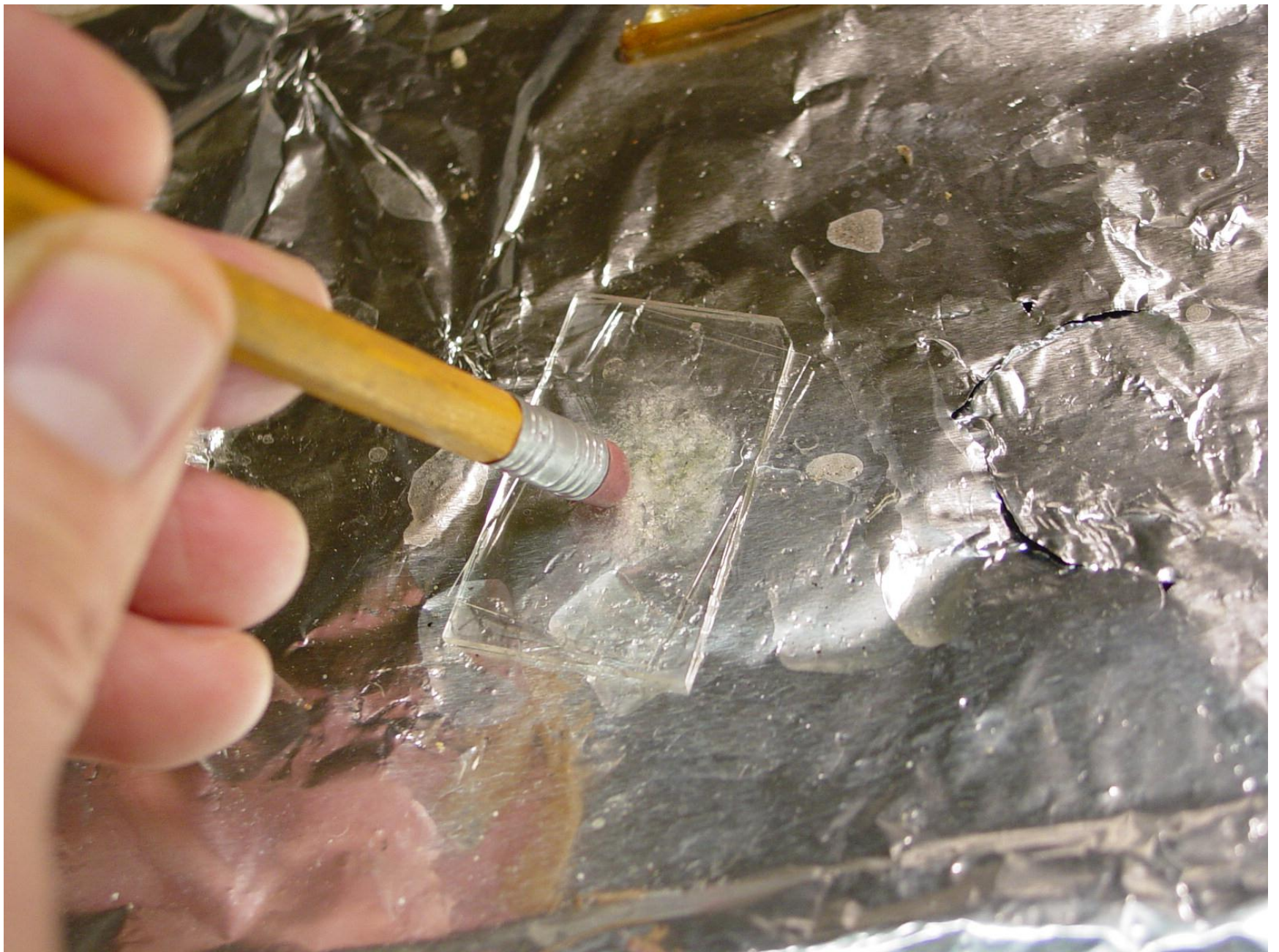
Moving cover slip to spread epoxy and expel bubbles.
