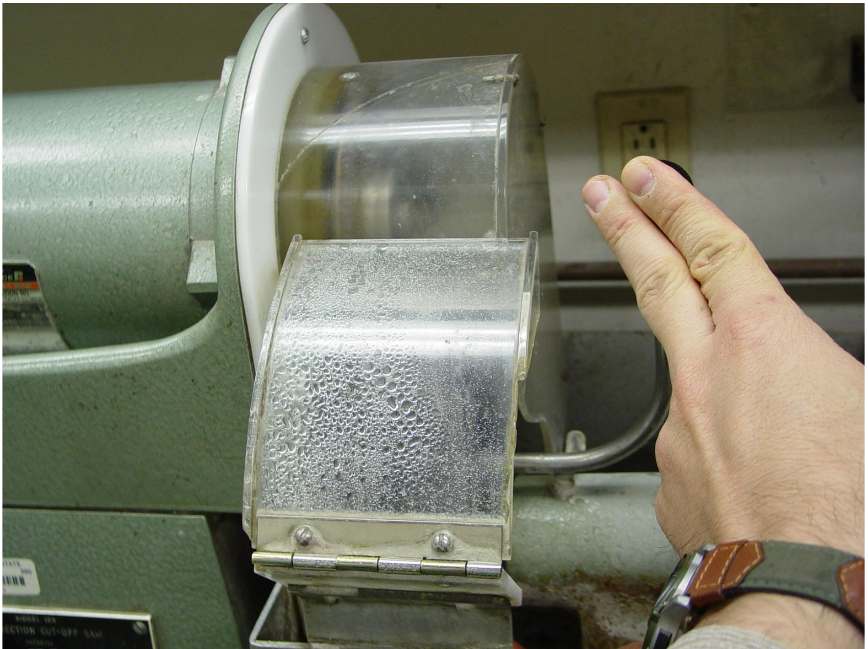
Slowly cutting off the chip from the slide.
