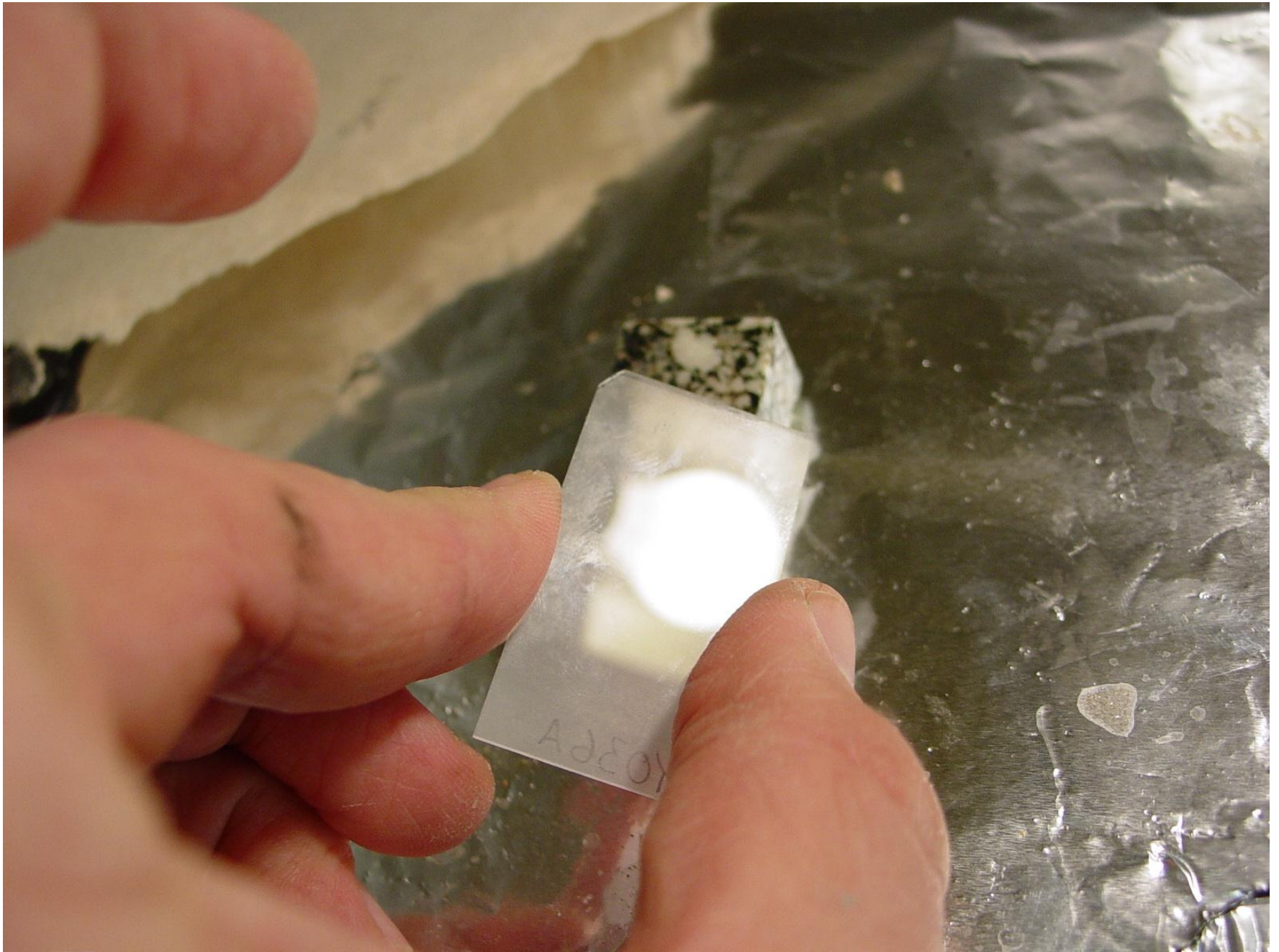
Placing slide on chip, frosted side down.
