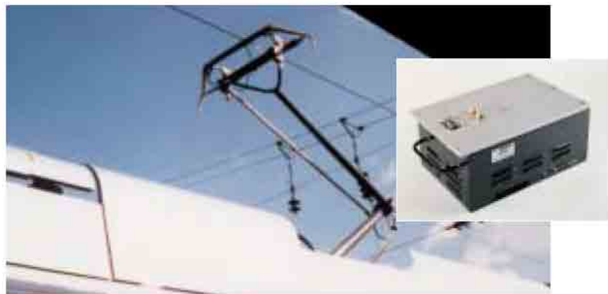
The ergonomic IPCU block is housed under the roof near the pantograph
