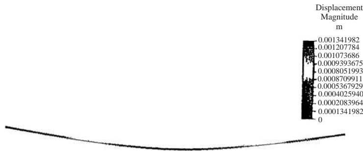
Figure 1: 400mm beam deflection with shear area included
