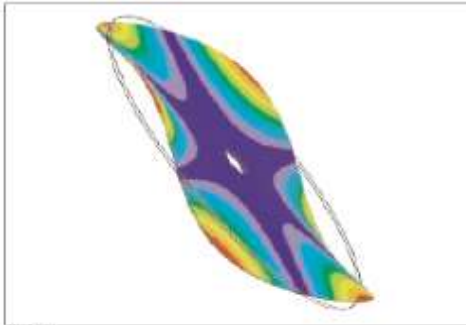
Figure 3 View of the higher stress regions of the hot case
