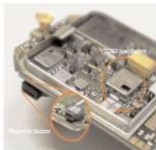
Figure 1: Circuit board of a multi-phase.
