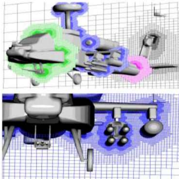
Upper: Cartesian mesh for attack helicopter configuration with 5.81M cells, Lower: Close-up of mesh through left wing and stores.
