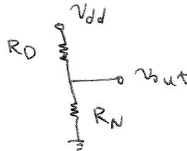
$$R_N = g_{m1} r_{o1} R_S + r_{o1} + R_S, \quad \frac{V_{out}}{V_{DD}} = \frac{R_N}{R_N + R_D}$$
