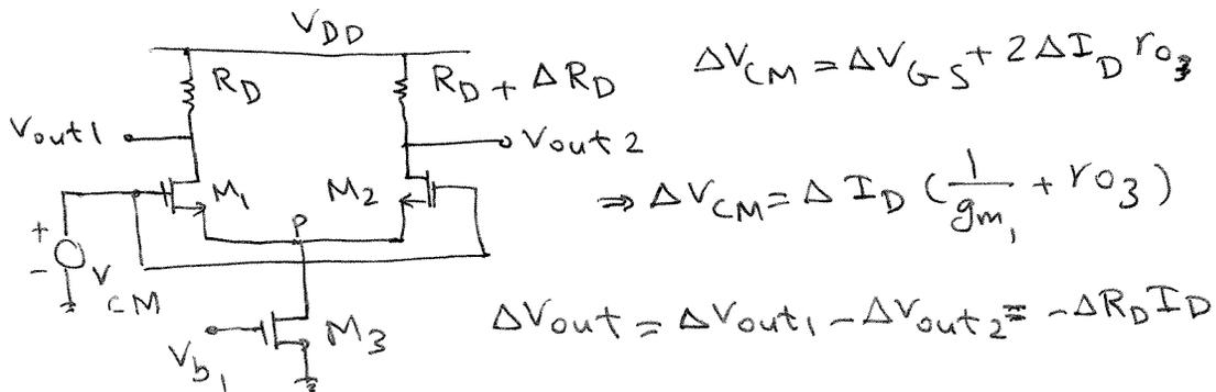
$$\Rightarrow A_{CM,DM} = \frac{\Delta V_{out}}{\Delta V_{CM}} = - \frac{\Delta R_D / 2}{\frac{1}{2g_{m1}} + r_{o3}}$$
