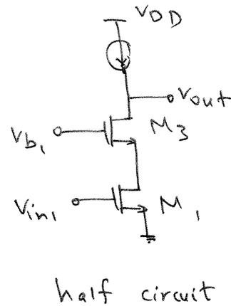
$$A_v = 300, \quad W/L = \frac{20}{0.18}, \quad \mu_n C_{ox} = 100 \mu\text{A}/\text{V}^2$$
