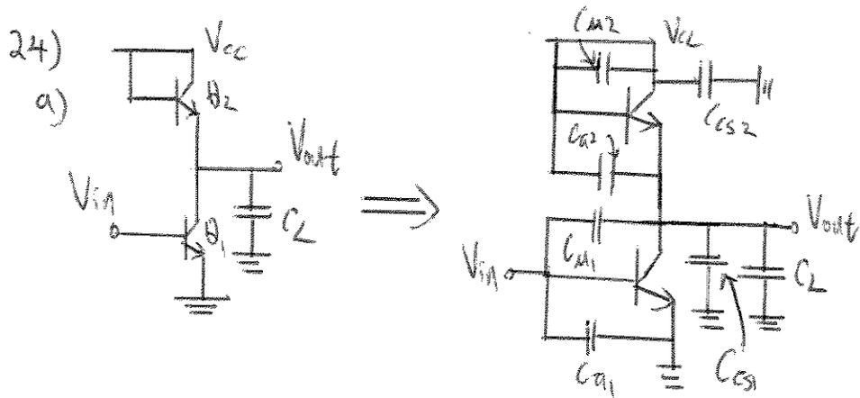
$C_{M2}$ ,  $C_{S1}$ ,  $C_L$  are in parallel
