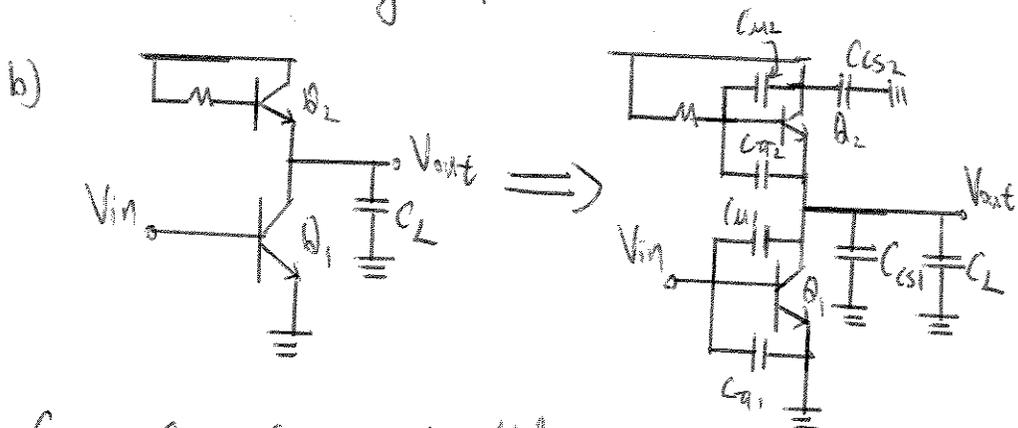
$C_{S1}$ ,  $C_L$  are in parallel
