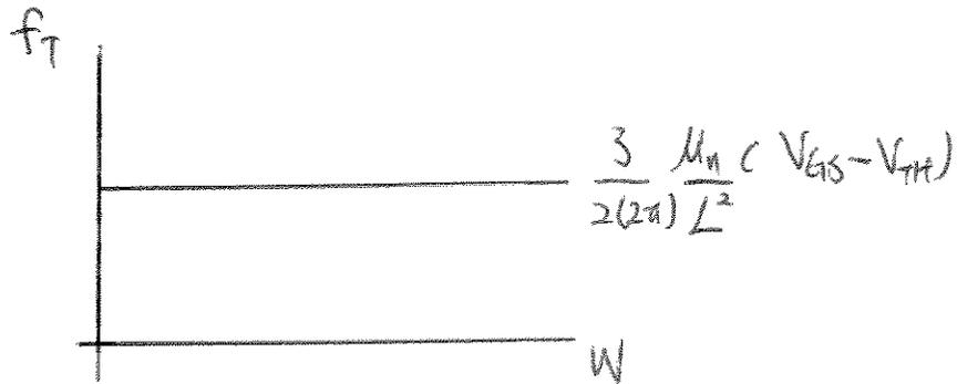
b) Using equation  $2\pi f_T = \frac{3}{2} \frac{\mu_n}{L^2} (V_{GS} - V_{TH})$ ,
