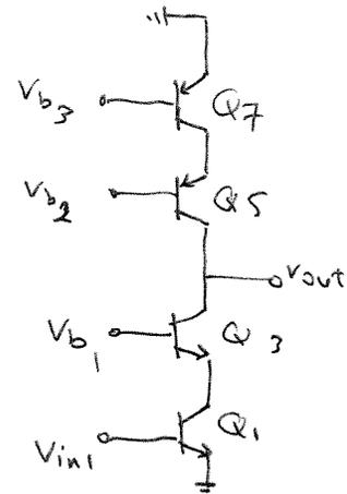
$$A_V = 800, \quad \beta_n = 2\beta_p = 100, \quad V_{A,n} = 2V_{A,p}$$
