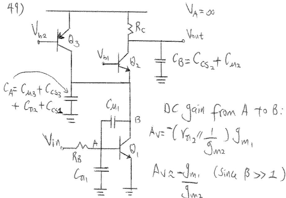
We have  $I_{C2} = 0.25 I_{C1}$ ,  $g_m = \frac{I_C}{V_T} \Rightarrow g_{m2} = 0.25 g_{m1}$
