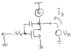
$$Z_{out} = \frac{V_x}{\bar{i}_x} = \frac{1 + sC_F R_G}{sC_F (1 + g_{m1} R_G)}$$
