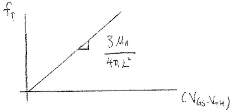
b) Using equation  $2\pi f_T = \frac{3\mu_n}{2L^2} (V_{GS} - V_{TH})$
