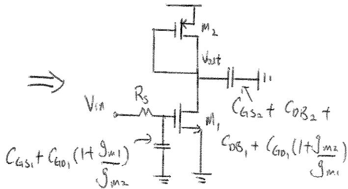
$$\text{DC gain} = -g_{m1} (V_{o1} // V_{o2} // \frac{1}{g_{m2}}) \approx -\frac{g_{m1}}{g_{m2}}$$
