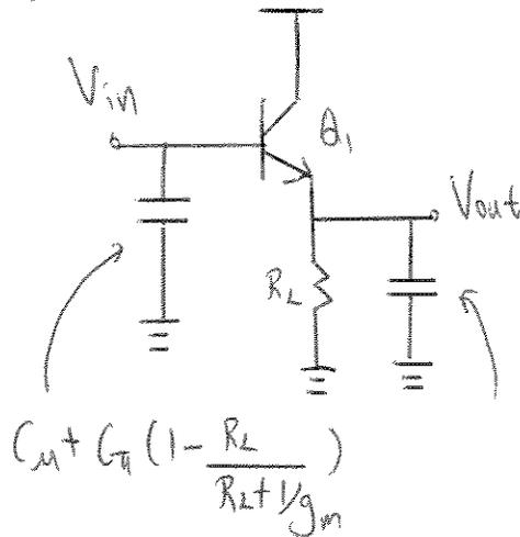
$$\text{DC gain: } \frac{R_L}{R_L + 1/g_m}$$
