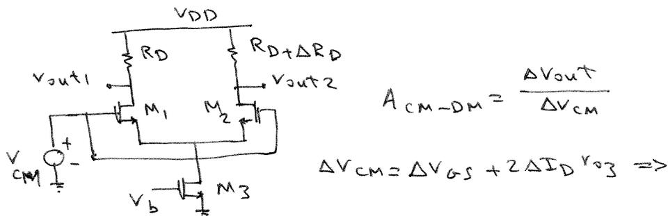
$$\Delta V_{cm} = \Delta I_D \left( \frac{1}{g_{m1}} + 2r_{o3} \right)$$
