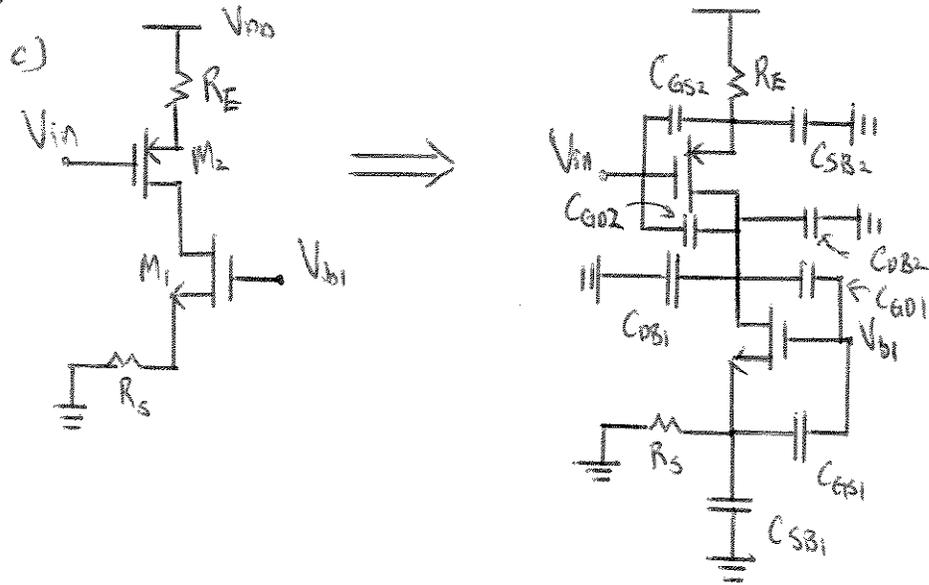
$C_{DB2}$ ,  $C_{GD1}$ ,  $C_{DB1}$ , are in parallel
