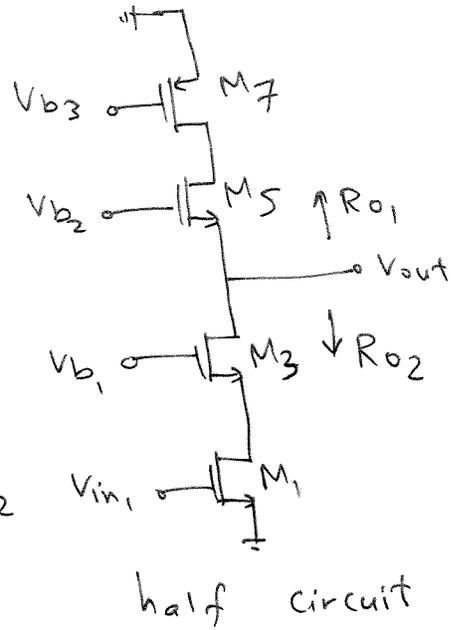
$$R_{o2} = g_{m3} r_{o3} r_{o1} + r_{o1} + r_{o3}$$
