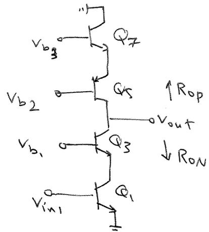
$$R_{ON} = (r_{o1} \parallel r_{\pi 3}) + r_{o3} + g_{m3} r_{o3} (r_{o1} \parallel r_{\pi 3})$$
