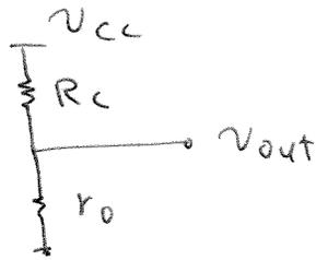
$$\frac{v_{out}}{v_{CC}} = \frac{r_o}{r_o + R_C} = \frac{\frac{V_A}{I_C}}{\frac{V_A}{I_C} + R_C} = \frac{V_A}{V_A + R_C I_C}$$
