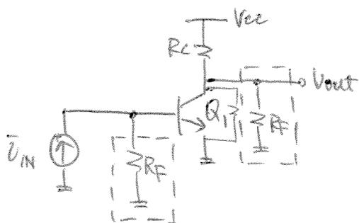
This is the open-loop circuit with consideration of I/O loading.
