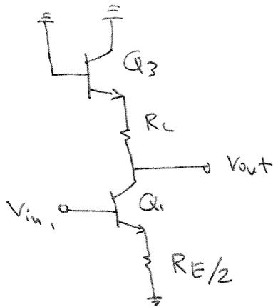
$$a) A_v = \frac{v_{out}}{v_{in1}} = - \frac{R_c + 1/g_{m3}}{R_{E/2} + 1/g_{m1}}$$
