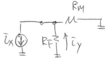
$$A_{CL} = \frac{A_I}{1 + A_I K} = \frac{g_{m2} R_C}{1 + g_{m2} R_C \frac{(R_F \parallel R_M)}{R_F}}$$
