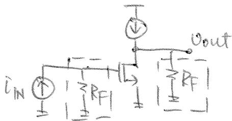
$$R_{o.L.} = \frac{V_{out}}{i_{IN}} = -g_m R_F R_F = -g_m R_F^2$$
