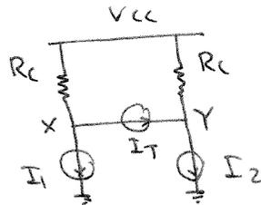
$$V_x = V_{cc} - R_c (I_1 + I_T) = V_{cc} - R_c (I_0 + I_T) - R_c I_0 \cos \omega t$$
