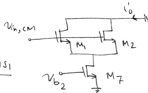
$$G_m = \frac{i'_o}{v_{in,CM}} = \frac{2g_{m1} v_{gs1}}{v_{in,CM}}$$
