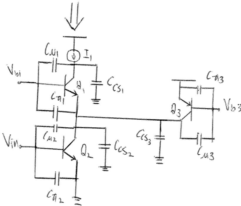
$C_{\mu 1}, C_{CS2}, C_{CS3}, C_{\mu 3}$  are in parallel
