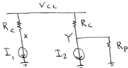
$$V_x = V_{CC} - R_c I_1 = V_{CC} - R_c I_0 (1 + \cos \omega t)$$
