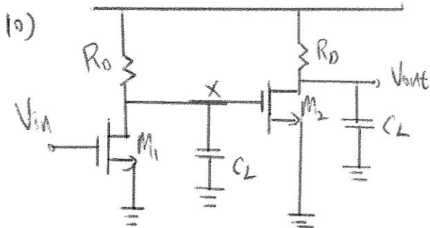
$$\frac{V_x(s)}{V_{in}} = -g_m \left( R_D \parallel \frac{1}{C_L s} \right), \quad \frac{V_{out}(s)}{V_x} = -g_m \left( \frac{R_D}{R_D C_L s + 1} \right)$$
