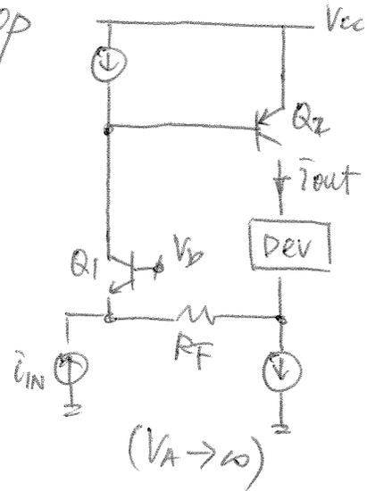
$$A_{I, o.l.} = \frac{i_{out}}{i_{in}} = \frac{i_{out}}{v_x} \times \frac{v_x}{i_{in}}$$
