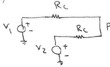
$$V_P = \frac{V_1 + V_2}{2} = V_0$$
