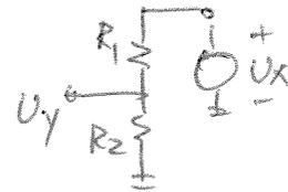
$$R_{in, OPEN} = \frac{r_{\pi 1} + (R_1 \parallel R_2)}{\beta_1 + 1} \approx \frac{1}{g_{m1}} + \frac{R_1 \parallel R_2}{\beta_1 + 1}$$
