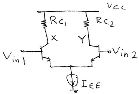
$$\begin{aligned}A_v &= 10, \\ P &= 2 \text{ mW} \\ V_{CC} &= 2.5 \text{ V} \\ V_A &= \infty\end{aligned}$$
