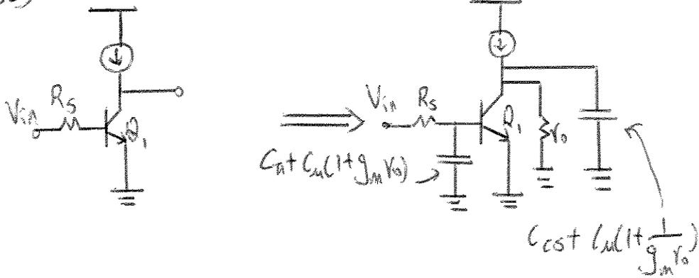
$$\omega_{p1} = \frac{1}{(R_s \parallel r_{\pi}) [C_{\pi} + C_{\mu}(1 + g_m R_o)]}$$
