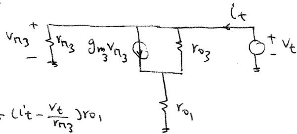
$$v_t = (i_t - g_{m3} v_t - \frac{v_t}{r_{\pi 3}}) r_{o3} + (i_t - \frac{v_t}{r_{\pi 3}}) r_{o1}$$
