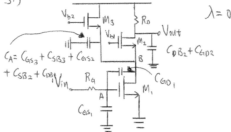
$$\text{DC gain from A to B: } -g_{m1} \left( \frac{1}{g_{m3}} \parallel \frac{1}{g_{m2}} \right) = -g_{m1} \left( \frac{1}{g_{m2} + g_{m3}} \right)$$
