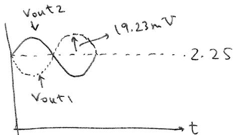
(b)  $I_{C1} = 0.95 I_{EE}$ ,  $I_{C2} = 0.05 I_{EE}$ ,  $\frac{I_{C1}}{I_{C2}} = 19$
