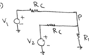
$$\frac{2V_P - V_1 - V_2}{R_c} + \frac{V_P}{R_i} = 0 \Rightarrow$$
