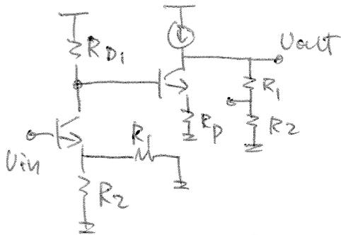
$$A_{OL} \cong \frac{-g_{m1} \times \{R_{D1} \parallel [\Gamma_{\pi 2} + (\beta_2 + 1)R_p]\}}{1 + g_{m1}(R_1 \parallel R_2)} \times \frac{-g_{m2}(R_1 + R_2)}{1 + g_{m2}R_p}$$
