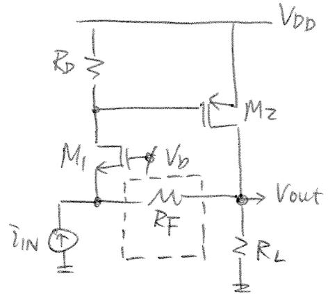
$$r_{out} \approx R_L \quad (R_F \text{ large})$$
