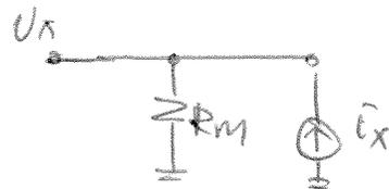
$$\therefore G_{o.l.} = \frac{G_{o.l.}}{1 + G_{o.l.} \times K} = \frac{G_{o.l.}}{1 + G_{o.l.} \times R_M}$$
