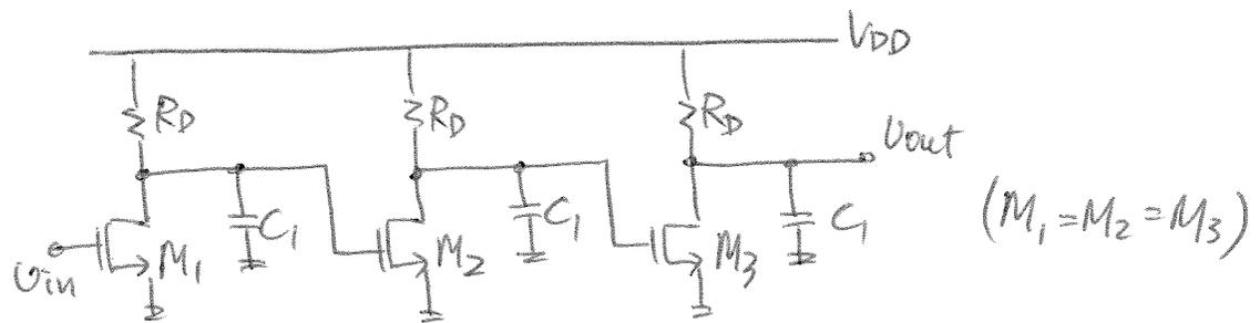
$$H(s) = \frac{V_{out}}{V_{in}}(s) = \frac{(-g_m R_D)^3}{\left(1 + \frac{s}{\omega_p}\right)^3} \quad \text{where } \omega_p = \frac{1}{R_D C_1}$$
