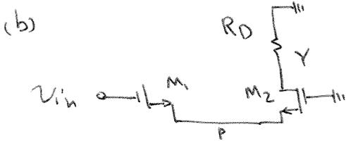
$$v_p = \frac{\frac{1}{g_{m2}}}{\frac{1}{g_{m1}} + \frac{1}{g_{m2}}} v_{in}$$
