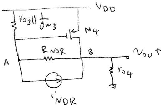
$$\begin{cases} \frac{V_A - V_B}{R_{NOR}} + \frac{V_A}{r_{o3} \parallel \frac{1}{g_{m3}}} + i_{NOR} = 0 \Rightarrow V_A = \frac{\frac{V_B}{R_{NOR}} - i_{NOR}}{\frac{1}{R_{NOR}} + \frac{1}{r_{o3} \parallel \frac{1}{g_{m3}}}} \\ \frac{V_B - V_A}{R_{NOR}} + \frac{V_B}{r_{o4}} - i_{NOR} + g_{m4} V_A = 0, V_B = v_{out} \end{cases}$$
