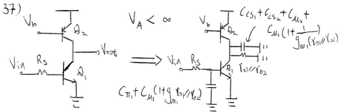
$$\omega_{pin} = \frac{1}{(R_s/V_{in}) [C_{\pi 1} + C_{\mu 1} (1 + g_{m1} (V_{o1}/V_{o2}))]}$$
