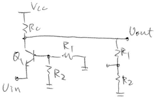
$$A_{OL} \approx g_{m1} [R_c \parallel (R_1 \parallel R_2)] \quad \text{since } \bar{v}_b \rightarrow 0 \quad (\beta \gg 1)$$
