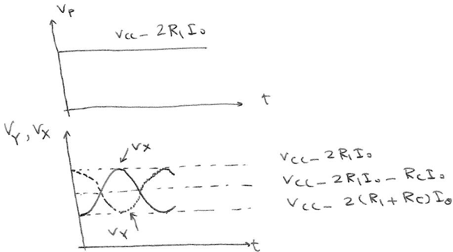
$$V_{X,CM} = V_{Y,CM} = V_{CC} - (2R_1 + R_C) I_0$$
