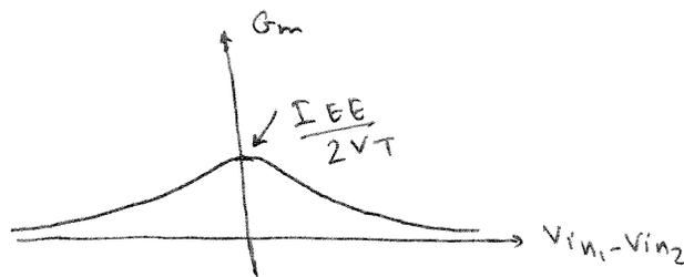
$$\begin{cases} \max G_m = \frac{I_{EE}}{2V_T} \\ \text{At } v_{in1} - v_{in2} = 0 \end{cases}$$
