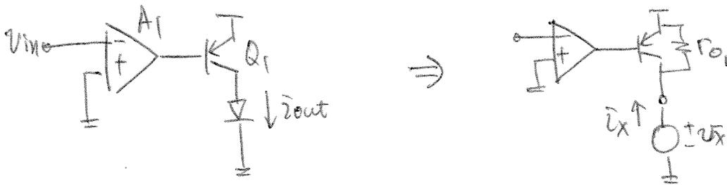
$$\therefore R_{out, OPEN} = \frac{V_x}{i_x} = r_{o1}$$
