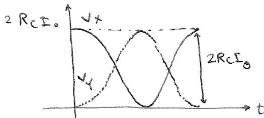
$$V_{X,P-P} = V_{Y,P-P} = 2R_C I_0$$
