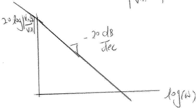
For an integrator, the gain at arbitrary low freq approaches infinity.
