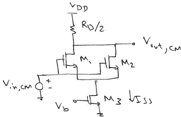
$$g_{m1} = g_{m2} = \frac{2 I_{SS}/2}{(V_{GS} - V_{TH})_{eq}}$$
