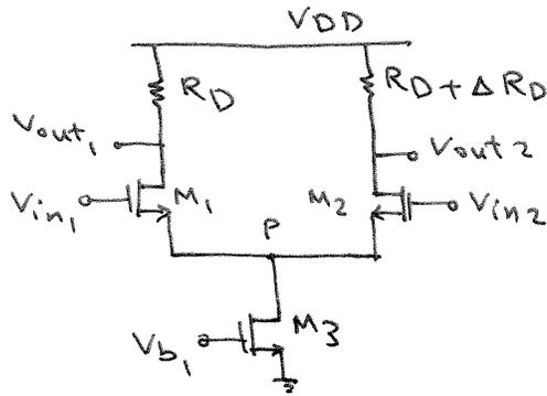
To calculate  $A_{DM}$ , using the half circuit:
