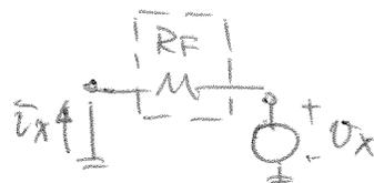
$$\therefore R_{o.L.} = \frac{R_{o.L.}}{1 + R_{o.L.} \times K} = \frac{-g_m(R_F \parallel r_{\pi})(R_C \parallel R_F \parallel r_o)}{1 + \frac{g_m(R_F \parallel r_{\pi})(R_C \parallel R_F \parallel r_o)}{R_F}}$$
