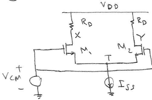
$$V_T = V_{CM} - V_{GS1} = V_{CM} - V_{TH} - \sqrt{\frac{I_{SS}}{\mu_n C_{ox} \frac{W}{L}}}$$
