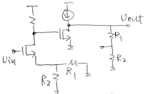
$$A_{OL} = \frac{-g_{m1} R_{D1}}{1 + g_{m1}(R_1 \parallel R_2)} \times -g_{m2}(R_1 + R_2)$$
