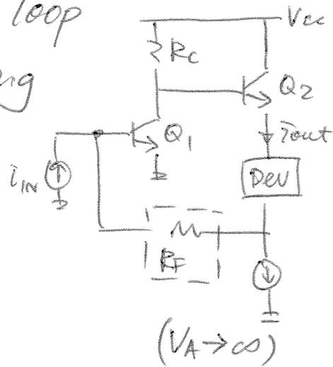
$$A_{I,OL} = \frac{i_{out}}{i_{in}} = \frac{i_{out}}{u_x} \times \frac{u_x}{i_{in}}$$
