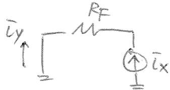
$$\Rightarrow A_{I, c.l.} = \frac{A_{I, o.l.}}{1 + A_{I, o.l.} \times K} = \frac{A_{I, o.l.}}{1 - A_{I, o.l.}}$$
