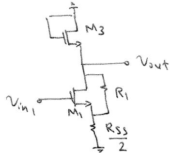
$$R_{out} = (r_{o3} \parallel \frac{1}{g_{m3}}) \parallel (g_{m1} (R_1 \parallel r_{o1}) \frac{R_{SS}}{2} + \frac{R_{SS}}{2} + R_1 \parallel r_{o1})$$
