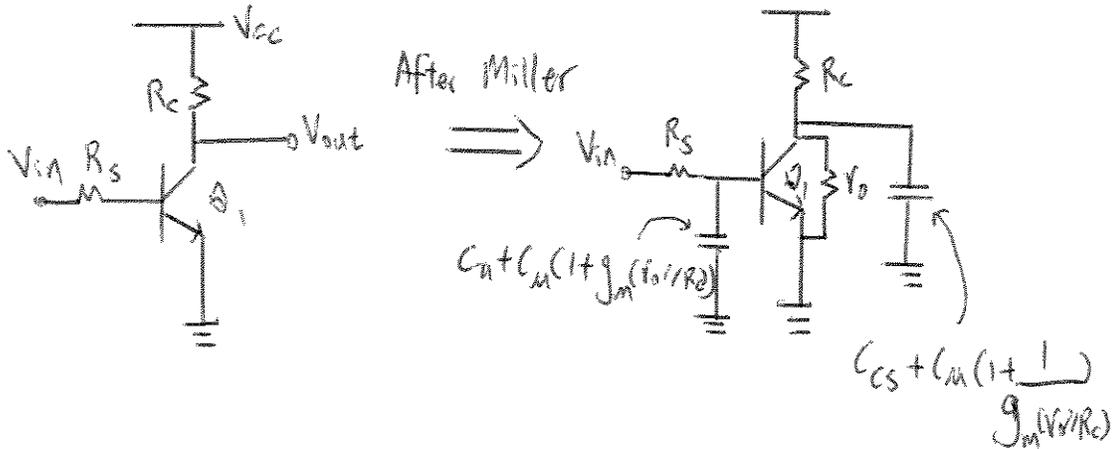
$$\omega_{p_{in}} = \frac{1}{(R_s // R_{in}) [C_c + C_c(1 + g_m(V_o/R_L))]}$$
