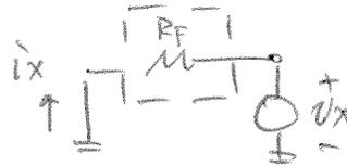
$$\Rightarrow R_{c.l.} = \frac{R_{o.l.}}{1 + R_{o.l.} \times k} = \frac{-g_{m1} g_{m2} R_D R_F \left( \frac{1}{g_{m1}} \parallel R_F \right)}{1 + g_{m1} g_{m2} R_D \left( \frac{1}{g_{m1}} \parallel R_F \right)}$$
