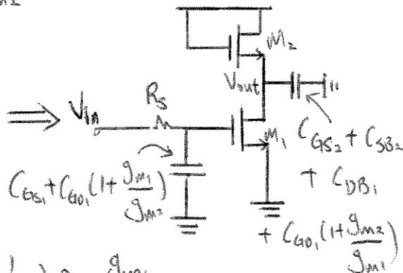
$$\text{DC gain} = -g_{m1} (V_{o1} // V_{o2} // \frac{1}{g_{m2}}) \approx -\frac{g_{m1}}{g_{m2}}$$
