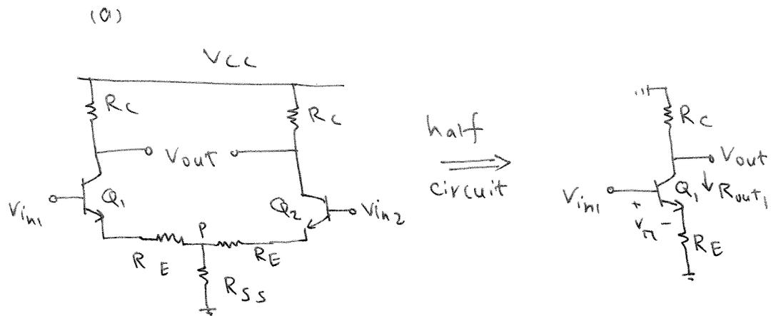
$$R_{out} = R_C \parallel R_{out1} = R_C \parallel (g_{m1} r_{o1} (R_E \parallel r_{\pi1}) + r_{o1} + (R_E \parallel r_{\pi1}))$$
