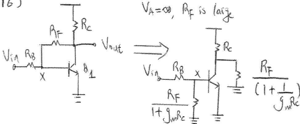
$$R_x = R_B \parallel \left( \frac{R_F}{1 + g_m R_c} \right), \quad R_{out} = R_c \parallel \left( \frac{R_F}{1 + \frac{1}{g_m R_c}} \right)$$
