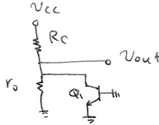
$$\frac{V_{out}}{V_{CC}} = \frac{r_o}{r_o + R_C} = \frac{V_A}{V_A + R_C I_{EE}}$$
