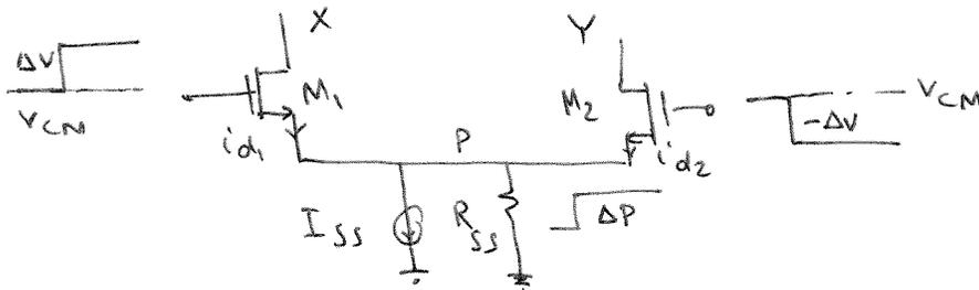
if  $V_{in1}$  and  $V_{in2}$  change by  $\Delta V$  and  $-\Delta V$  we have:
