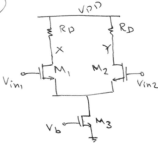
The same value for the inputs common-mode leads to the following circuit:
