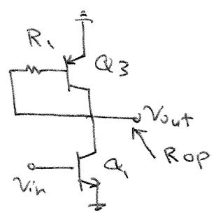
To calculate  $R_{op}$ , from small signal model we have:
