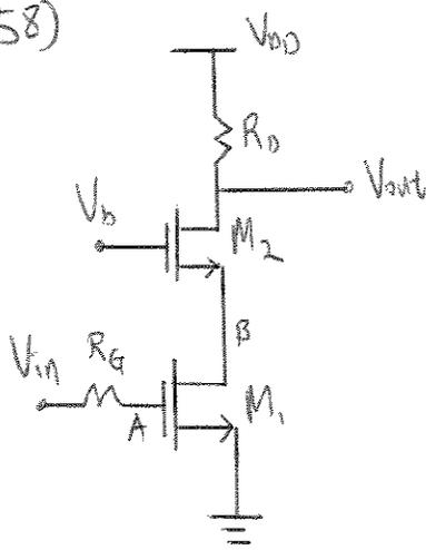
$$\begin{aligned} \omega_{pin} &= 5 \text{ GHz}, \quad \omega_{pout} = 10 \text{ GHz} \\ V_{eff} &= 200 \text{ mV} (V_{GS} - V_{th}), \quad I_D = 0.5 \text{ mA} \\ \lambda &= 0, \quad C_{GS} = (2/3) W L C_{ox}, \\ L &= 0.18 \mu\text{m}, \quad \mu_n C_{ox} = 100 \mu\text{A/V}^2 \\ C_{GD} &= W C_o, \quad C_o = 0.2 \text{ fF}/\mu\text{m} \\ C_{ox} &= 12 \text{ fF}/\mu\text{m}^2 \end{aligned}$$
