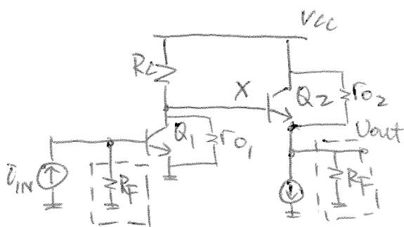
This is the open-loop circuit with consideration of I/O loading.
