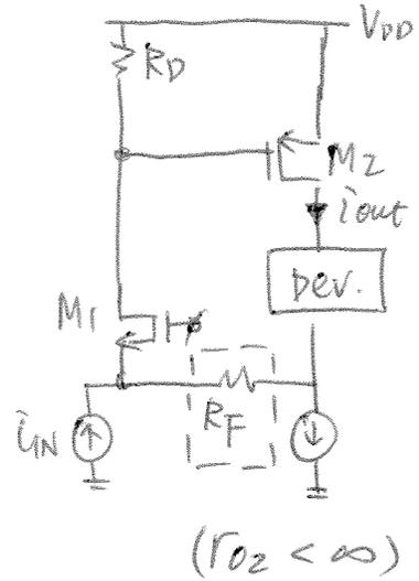
$$A_{I, o.l.} = \frac{\bar{i}_{out}}{\bar{i}_{in}} = \frac{\bar{i}_{out}}{V_x} \times \frac{V_x}{\bar{i}_{in}}$$
