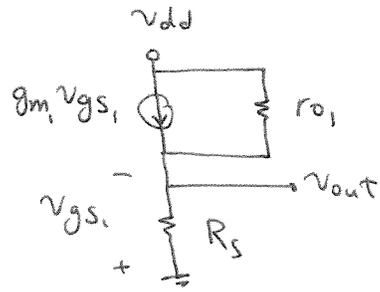
$$\frac{v_{out}}{R_S} + \frac{v_{out} - v_{dd}}{r_{o_1}} + g_m v_{out} = 0$$
