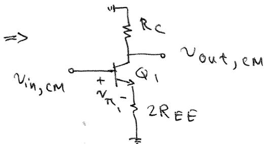
$$v_{out,cm} = -g_{m1} v_{\pi_1} R_c = -g_{m1} R_c \frac{\frac{1}{g_{m1}}}{\frac{1}{g_{m1}} + 2R_{EE}} v_{in,cm}$$
