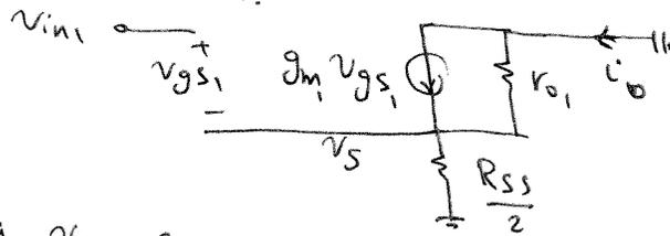
$$\frac{v_s}{r_{o1} \parallel \frac{R_{SS}}{2}} + g_{m1} v_s = g_{m1} v_{in} \Rightarrow v_s = \frac{g_{m1} v_{in}}{g_{m1} + \frac{1}{\frac{R_{SS}}{2} \parallel r_{o1}}}$$
