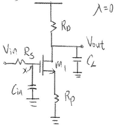
$$R_x = R_S, \quad R_{out} = R_D$$
