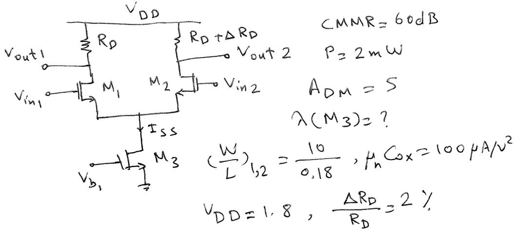
$$P = 2mW = I_{SS} V_{DD} \Rightarrow I_{SS} = \frac{2 \times 10^{-3}}{1.8} = 1.11 mA$$
