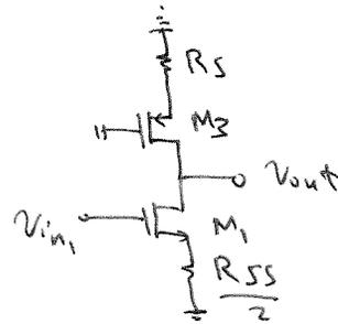
$$R_{out} = (g_{m3} r_{o3} R_s + r_{o3} + R_s) \parallel \left( g_{m1} r_{o1} \frac{R_{SS}}{2} + r_{o1} + \frac{R_{SS}}{2} \right)$$
