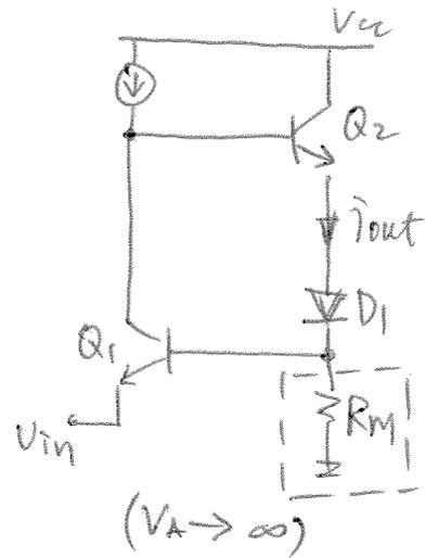
$$G_{o.L.} = \frac{i_{out}}{v_{in}} = \frac{i_{out}}{v_x} \times \frac{v_x}{v_{in}} \approx \frac{g_{m2}(R_L + R_M)}{1 + g_{m2}(R_L + R_M)} \times g_{m1} [\tau_{\pi 2} + (\beta_2 + 1)(R_L + R_M)]$$
