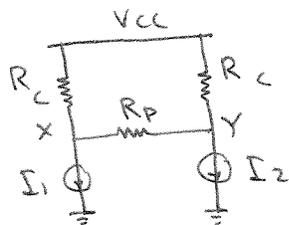
$$\begin{cases} \frac{V_x - V_{cc}}{R_c} + \frac{V_x - V_y}{R_p} + I_1 = 0 \\ \frac{V_y - V_{cc}}{R_c} + \frac{V_y - V_x}{R_p} + I_2 = 0 \end{cases} \Rightarrow$$
