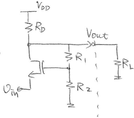
$$\text{Gain}_{\text{unloaded}} \cong \frac{g_m R_D}{1 + \frac{R_2}{R_1 + R_2} g_m R_D} \quad (\text{assume } R_1 + R_2 \gg R_D)$$
