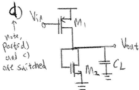
$$R_{out} = \frac{1}{g_{m2} \parallel Y_{o2} \parallel Y_{o1}} \approx \frac{1}{g_{m2}}$$
