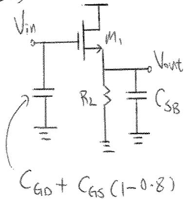
$$R_L = 100\Omega, \quad I_D = 1\text{mA}$$
