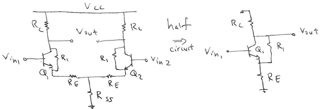
$$R_{out} = R_C \parallel \left( g_{m_1} (r_{o_1} \parallel R_1) (R_E \parallel r_{\pi_1}) + (r_{o_1} \parallel R_1) + (R_E \parallel r_{\pi_1}) \right)$$
