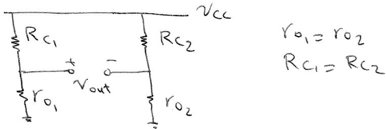
$$\frac{V_{out}}{V_{cc}} = \frac{1}{V_{cc}} \left( \frac{r_{o1}}{R_{C1} + r_{o1}} - \frac{r_{o2}}{R_{C2} + r_{o2}} \right) V_{cc} = 0$$
