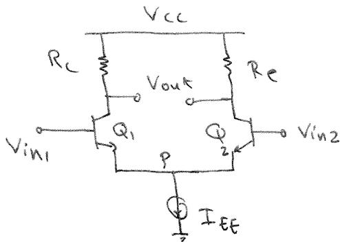
$$I_{C2} = \frac{I_{EE}}{1 + \exp\left(\frac{V_{in1} - V_{in2}}{V_T}\right)}$$
