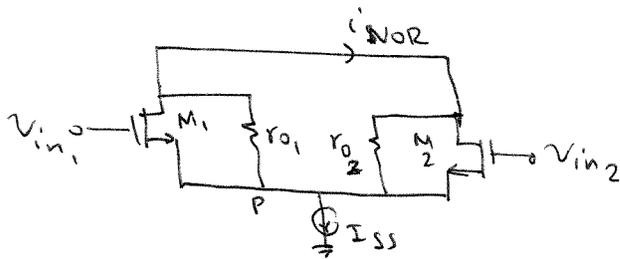
$$r_{o1} (i_{NOR} + g_{m1} v_{in1}) + r_{o2} (i_{NOR} - g_{m2} v_{in2}) = -I_{SS}$$
