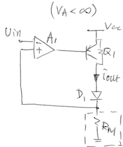
$$G_{OL} = \frac{\bar{i}_{out}}{U_{in}} = \frac{\bar{i}_{out}}{U_x} \times \frac{U_x}{U_{in}} \quad (1)$$
