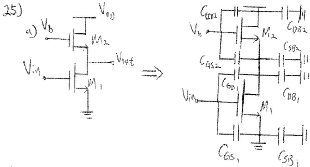
$C_{GS2}$ ,  $C_{SB2}$ ,  $C_{DB1}$  are in parallel
