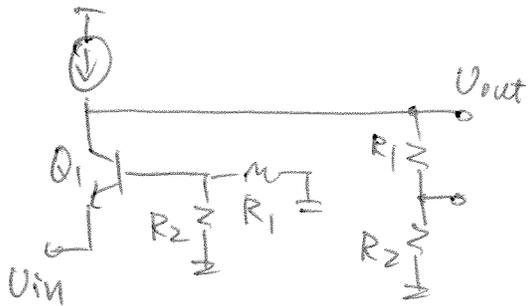
$$A_{OL} \cong g_{m1} (R_1 + R_2) \quad \text{since } i_b \rightarrow 0 (\beta \gg 1)$$
