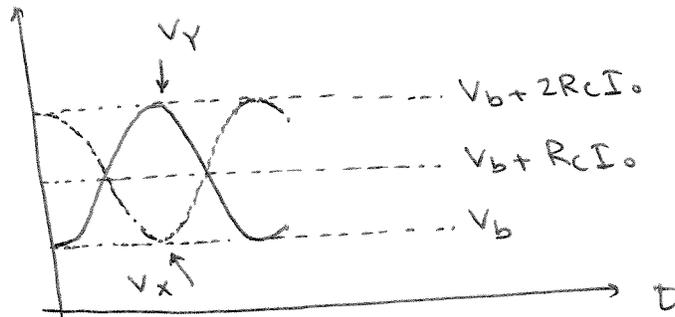
$$V_{X,CM} = V_{Y,CM} = V_b + R_C I_0$$
