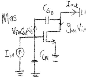
Similarly for MOS, with  $C_{\mu}$  and  $C_{\pi}$  replaced by  $C_{GD}$  and  $C_{GS}$  respectively.
