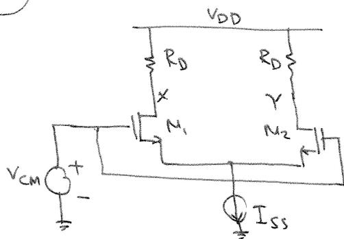
$$\begin{aligned}V_{CM} &= 1V \\ I_{SS} &= 1mA \\ R_D &= 1k\Omega\end{aligned}$$
