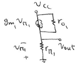
$$\frac{V_{out}}{r_{\pi 1}} + \frac{V_{out} - V_{CC}}{r_{o1}} + g_{m1} V_{out} = 0 \rightarrow (r_{\pi 1} + r_{o1} + g_{m1} r_{o1} r_{\pi 1}) V_{out} = \frac{r_{\pi 1}}{r_{\pi 1}} V_{CC}$$
