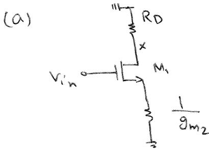
$$v_x = -g_{m1} v_{gs1} R_D =$$
