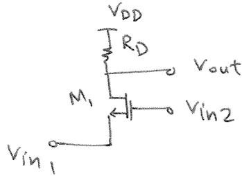
$$I_{D1} = \frac{1}{2} \mu_n C_{ox} \left(\frac{W}{L}\right) (V_{in2} - V_{in1} - V_{TH})^2$$
