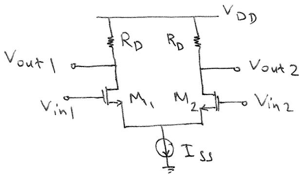
$$\begin{aligned} P &= 2 \text{ mW} \\ \text{overdrive} &= 100 \text{ mV} \\ V_{CM} &= 1 \text{ V} \\ \lambda &= 0, \mu_n C_{ox} = 100 \mu\text{A/V}^2 \\ V_{DD} &= 1.8 \text{ V} \\ V_{TH,n} &= 0.5 \end{aligned}$$
