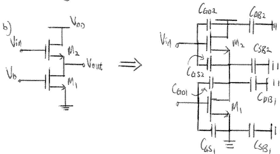
$C_{GD1}$ ,  $C_{DB1}$ ,  $C_{SB2}$  are in parallel
