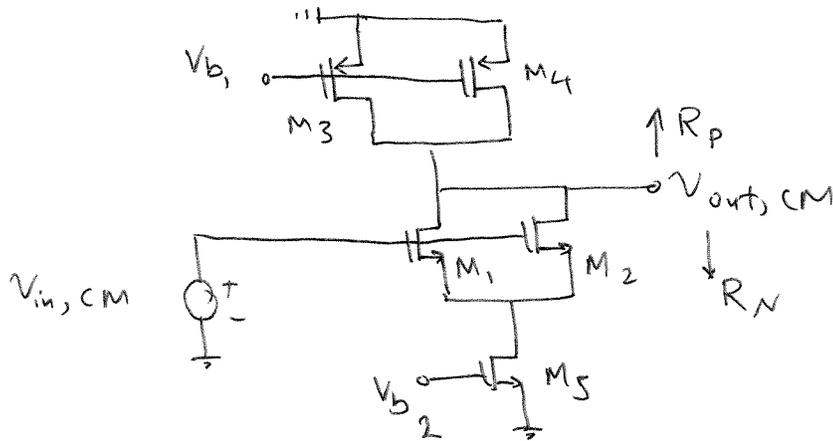
$$R_P = r_{o3} \parallel r_{o4} = \frac{r_{o3}}{2} = \frac{r_{o4}}{2}$$
