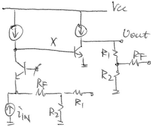
$$R_{OL} = \frac{U_{out}}{i_{IN}} = \frac{U_{out}}{U_X} \times \frac{U_X}{i_{IN}} = [-g_{m2}(R_1 + R_2)] \times [g_{m1}, r_{\pi 2} \left\{ \frac{1}{g_{m1}} \parallel (R_F + R_2) \right\}]$$
