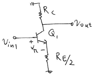
$$A_v = \frac{v_{out}}{v_{in1}} \approx \frac{-g_{m1} v_{\pi} R_C}{v_{in1}} = -\frac{g_{m1} R_C}{\frac{1}{g_{m1}} + \frac{R_E}{2}} v_{in1}$$
