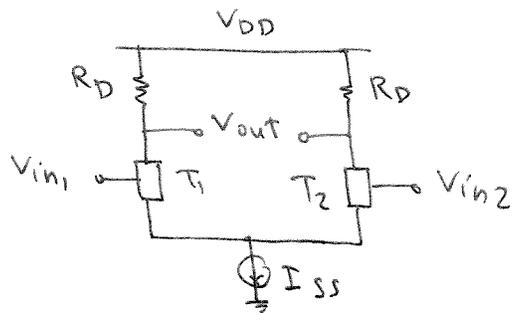
(a) The characteristic of  $I_{D1} - I_{D2}$  vs.  $V_{in1} - V_{in2}$  is similar to the standard CMOS differential pair, because it has saturation part.
