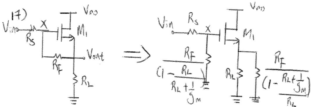
$$R_{out} = R_L \parallel \frac{R_F}{1 - \frac{R_L + \frac{1}{g_m}}{R_L}} = R_L \parallel \frac{R_F}{-\frac{1}{g_m R_L}}$$
