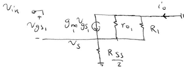
$$\frac{v_s}{\frac{R_{SS}}{2} \parallel R_1 \parallel r_{o1}} + g_{m1} v_s = g_{m1} v_{in} \Rightarrow v_s = \frac{g_{m1} v_{in}}{g_{m1} + \frac{1}{\frac{R_{SS}}{2} \parallel R_1 \parallel r_{o1}}}$$
