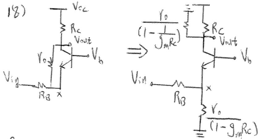
$$R_{out} = R_c \parallel \left( \frac{V_o}{1 - \frac{1}{g_m R_c}} \right)$$
