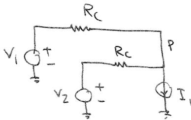
$$\frac{2V_P - V_1 - V_2}{R_c} + I_1 = 0 \Rightarrow$$
