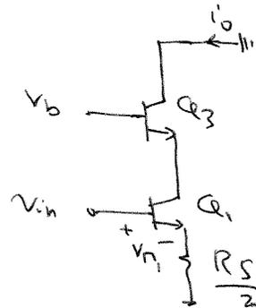
$$G_m = \frac{i_o}{v_{in}} = \frac{+g_{m1} v_{\pi 1}}{v_{in}} = \frac{+g_{m1}}{1 + g_{m1} \frac{R_s}{2}}$$
