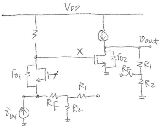
$$K = -\frac{(R_F \parallel R_2) / R_F}{R_F \parallel R_2 + R_1}$$
