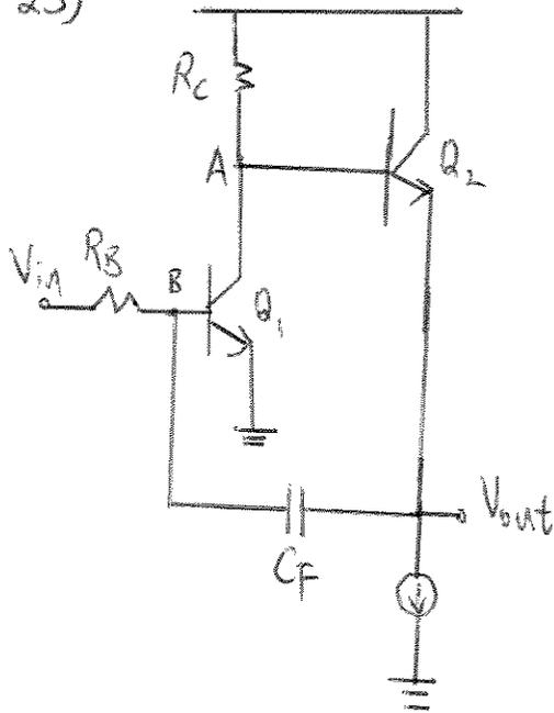
The gain from B to A is  $-g_m R_C$ , from A to out is 1 (since we have an ideal current source). So the gain from B to out is  $-g_m R_C$ .
