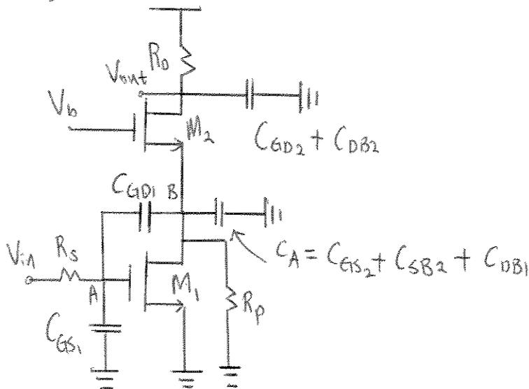
DC gain from A to B is  $-g_{m1} (R_p \parallel \frac{1}{g_{m2}})$
