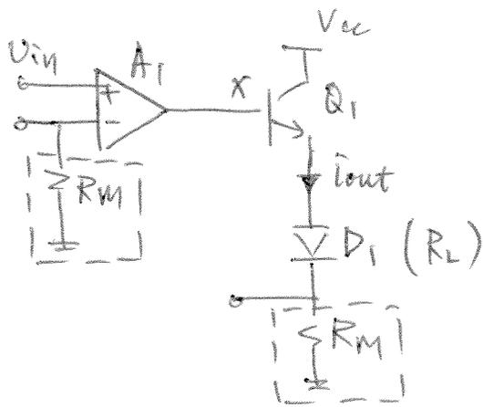
$$G_{o.l.} = \frac{i_{out}}{v_{in}} = \frac{i_{out}}{v_x} \cdot \frac{v_x}{v_{in}} = \frac{g_{m1} (R_L + R_M)}{1 + g_{m1} (R_L + R_M)} \times A_1$$
