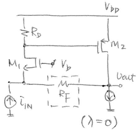
$$R_{o.l.} = \frac{v_x}{i_{in}} \cdot \frac{v_{out}}{v_x}$$
