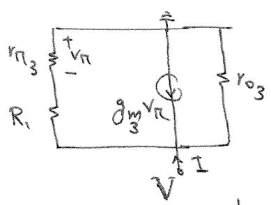
$$I = \frac{V}{r_{o3}} - g_{m3}V_{\pi} + \frac{V}{R_1 + r_{\pi 3}} = V \left[ \frac{1}{r_{o3}} + \frac{1}{R_1 + r_{\pi 3}} \right] + g_{m3} \frac{r_{\pi 3}}{R_1 + r_{\pi 3}} V$$
