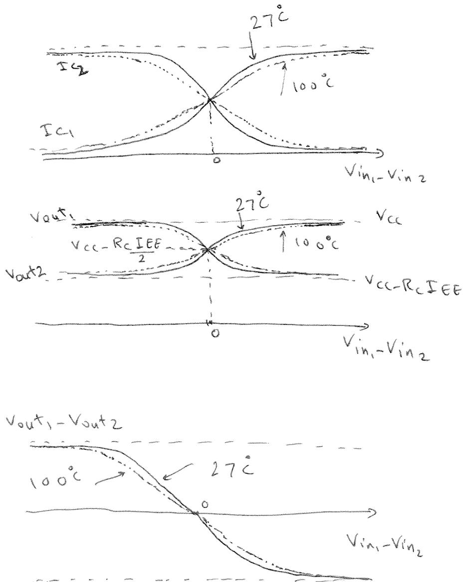
(24)  $R_C = 500 \Omega$ ,  $I_{EE} = 1 \text{ mA}$ ,  $V_{CC} = 2.5 \text{ V}$
