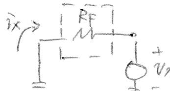
$$\Rightarrow R_{c.L.} = \frac{-g_m R_F^2}{1 + g_m R_F}$$
