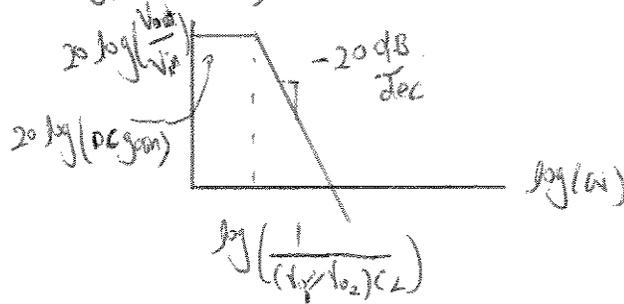
d)  $|DC \text{ gain}| = g_{m1} / g_{m2}$
