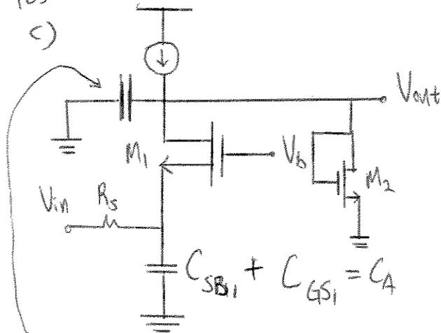
$$C_B = C_{DB1} + C_{GD1} + C_{DB2} + C_{GS2}$$
