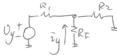
$$R_{OL} = \frac{v_{out}}{i_{IN}} = \frac{v_{out}}{v_x} \times \frac{v_x}{i_{IN}}$$
