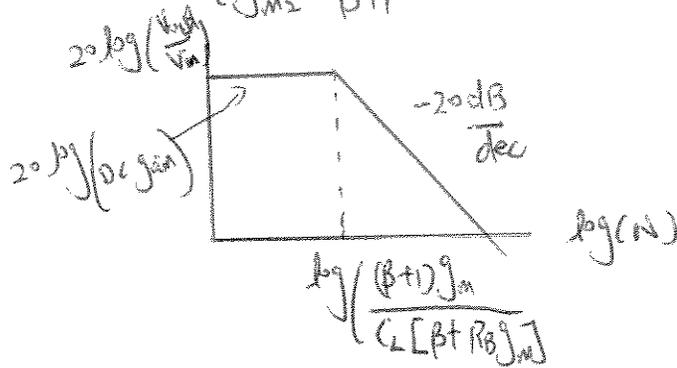
c)  $|DC \text{ gain}| = g_{m1} (R_{o1} / R_{o2})$
