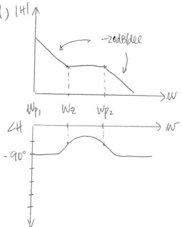
61. As  $\omega_z$  comes closer to  $\omega_{p1}$  or  $\omega_{p2}$ , it cancels out the effect (i.e.  $-20\text{dB/dec}$  decrease) — pole-zero cancellation. It would appear as if nothing occurred at that overlapping frequency.
