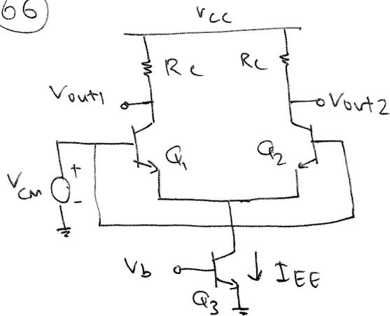
$$A_{cm} = \frac{\Delta V_{out, CM}}{\Delta V_{in, CM}} = \frac{R_c/2}{\frac{1}{2g_m} + r_{o3}} \Rightarrow$$
