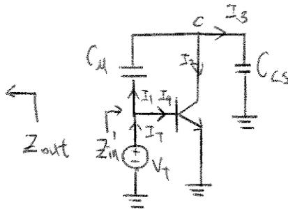
$$Z_{in} = Z_{in}' \parallel \frac{1}{C_{\pi} s}, \quad I_T = I_1 + I_4 = C_{\mu} s V_{bc} + \frac{g_m V_T}{\beta}$$
