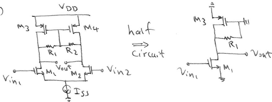
$$A_v = -g_{m1} (r_{o1} \parallel r_{o3} \parallel R_1)$$
