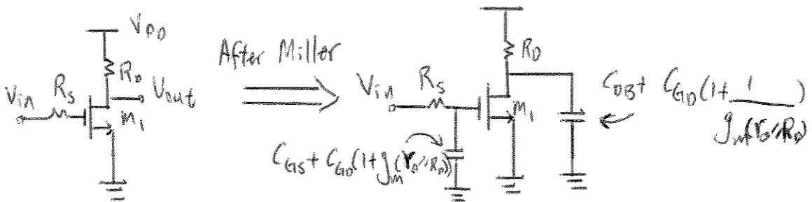
$$\omega_{p_{in}} = \frac{1}{R_s [C_{cs} + C_{cd}(1 + g_m(V_o/R_L))]}$$
