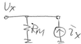
$$\Rightarrow G_{c.L.} = \frac{G_{o.L.}}{1 + G_{o.L.} \times k} = \frac{G_{o.L.}}{1 + G_{o.L.} R_M}$$
