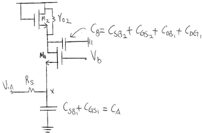
$$V_{out} = -(0 - V_x) g_{m1} \left[ \frac{1}{g_{m2}} \parallel \frac{1}{C_B s} \right] = V_x g_{m1} \left[ \frac{1}{g_{m2}} \parallel \frac{1}{C_B s} \right]$$
