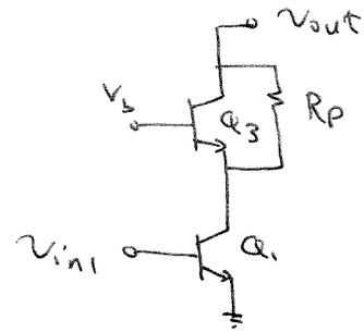
$$A_V = -g_{m1} (g_{m3} (r_{o3} \parallel R_P) (r_{o1} \parallel r_{\pi3}) + (r_{o3} \parallel R_P) + (r_{o1} \parallel r_{\pi3}))$$
