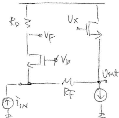
$$V_F = V_x \frac{g_{m1} R_D}{1 + g_{m2} (R_F + \frac{1}{g_{m1}})}$$
