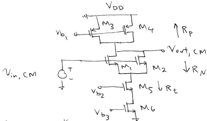
$$R_P = r_{o3} \parallel r_{o4} = \frac{r_{o3}}{2}$$
