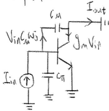
$$V_{in} = (I_{in}) \left( \frac{1}{[C_{\mu} + C_{\pi}] \omega j} \right) \quad (\text{Assuming we are at freq, and } V_A \text{ can be neglected})$$
