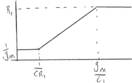
The bode-plot shows an impedance that increases with frequency, an inductive behavior.
