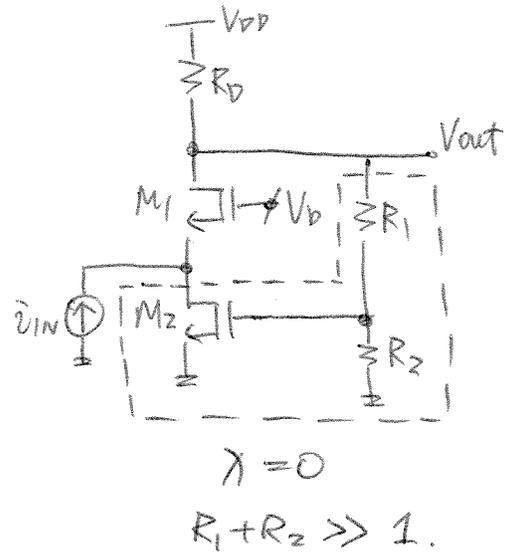
$$\Rightarrow R_{c.L.} = \frac{V_{out}}{\bar{v}_{IN}} = \frac{R_D}{1 + R_D \times g_{m2} \frac{R_2}{R_1 + R_2}}$$
