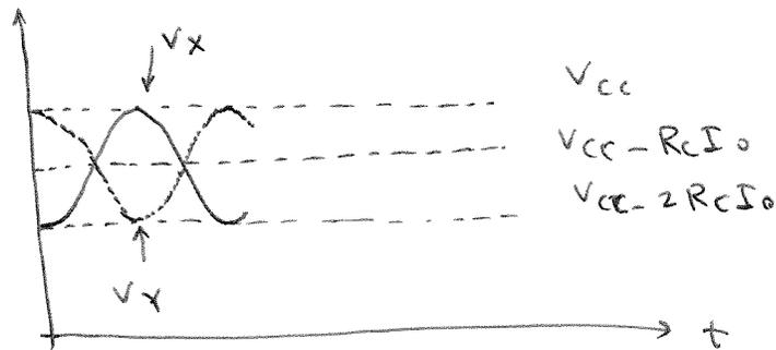
$$V_{X,CM} = V_{Y,CM} = V_{CC} - R_C I_0$$
