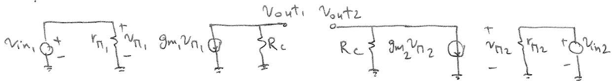
$$A_v = \frac{v_{out1} - v_{out2}}{v_{in1} - v_{in2}} = \frac{-g_{m1}v_{in1}R_C + g_{m2}v_{in2}R_C}{v_{in1} - v_{in2}} = -g_{m1}R_C$$
