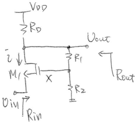
$$-V_{out} = \bar{i} [R_D \parallel (R_1 + R_2)]$$
