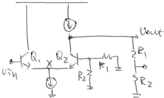
$$A_{OL} \cong \underbrace{\frac{g_{m1} \left( \frac{1}{g_{m2}} + \frac{R_1 || R_2}{\beta_2 + 1} \right)}{1 + g_{m1} \left( \frac{1}{g_{m2}} + \frac{R_1 || R_2}{\beta_2 + 1} \right)}}_{\text{emitter follower (Q}_1\text{)} = \frac{V_x}{V_{in}}} \times \underbrace{g_{m2} (R_1 + R_2)}_{\text{common-base stage (Q}_2\text{)} = \frac{V_{out}}{V_x}}$$
