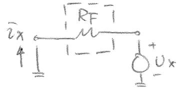
$$\therefore R_{o,L} = \frac{R_{o,L}}{1 + R_{o,L} \times k} = \frac{R_{o,L}}{1 - R_{o,L}/R_F}$$
