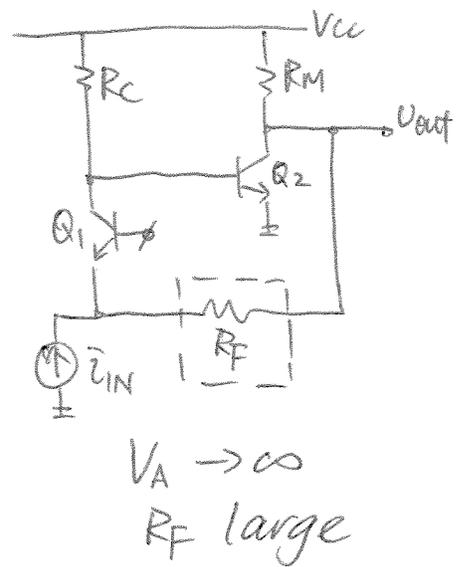
$$R_{OL} = \frac{v_{out}}{i_{IN}} = \frac{v_{out}}{v_X} \times \frac{v_X}{i_{IN}} \cong -g_{m2} R_M \times R_C$$
