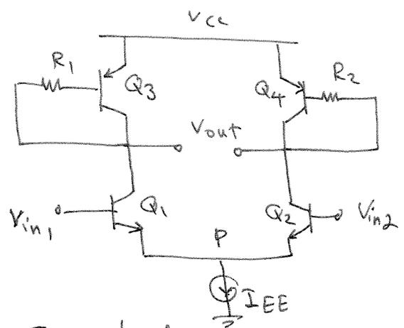
From half circuit concept we have:  $A_v = -g_{m1}(r_{o1} \parallel R_{op})$
