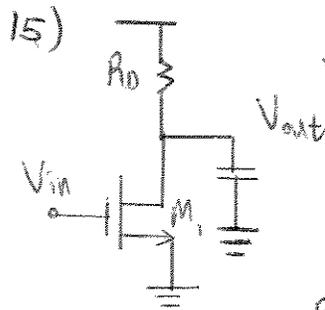
DC Gain:  $g_m R_D = \frac{2I_D R_D}{V_{eff}}$
