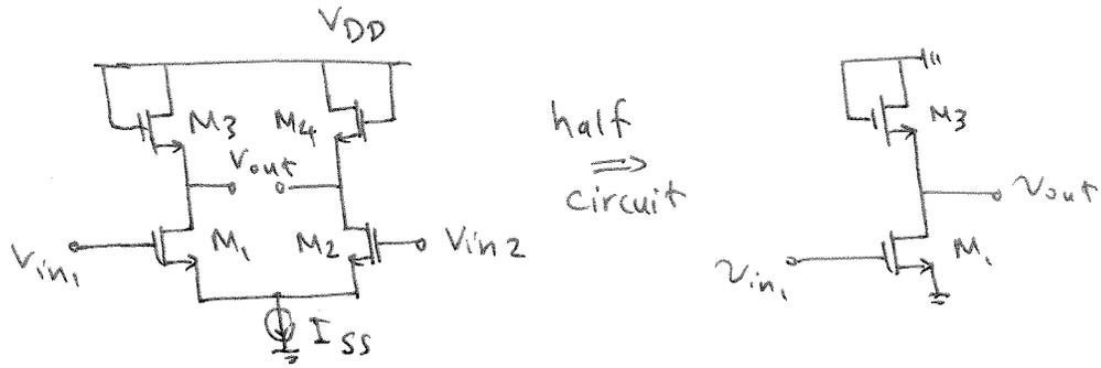
$$A_v = -g_{m1} (r_{o1} \parallel r_{o3} \parallel \frac{1}{g_{m3}})$$
