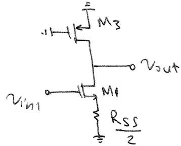
$$R_{out} = r_{o3} \parallel \left( g_{m1} r_{o1} \frac{R_{SS}}{2} + r_{o1} + \frac{R_{SS}}{2} \right)$$
