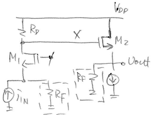
$$R_{in, OPEN} = \left( \frac{1}{g_{m1}} \parallel R_F \right)$$
