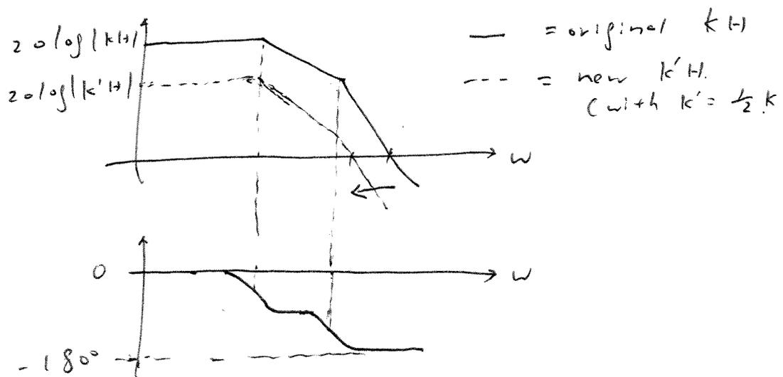
73) With the compensation capacitor  $C_c$  in place, the pole associated with  $C_c$  becomes dominant (i.e. at a lower frequency than the other 2 poles at  $\frac{1}{R_D C_1}$ ).
