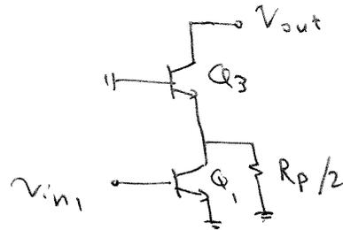
$$R_{out} = g_{m3} r_{o3} \left( \frac{R_p \parallel r_{o1} \parallel r_{o3}}{2} \right) + r_{o3} + \frac{R_p \parallel r_{o1} \parallel r_{o3}}{2}$$
