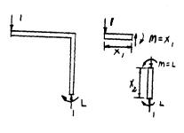
14-113. The L-shaped frame is made from two segments, each of length L and flexural stiffness EI. If it is subjected to the uniform distributed load, determine the horizontal displacement of the end C.
