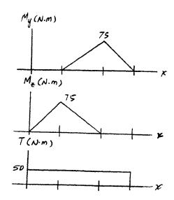
11-47 Determine to the nearest millimeter the diameter of the solid shaft if it is subjected to the gear loading. The bearings at A and B exert force components only in the y and z directions on the shaft. Base the design on the maximum-distortion-energy theory of failure with  $\sigma_{\rm allow} = 150$  MPa.
