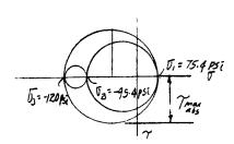
9-99 The crane is used to support the 350-lb load. Determine the principal stresses acting in the boom at points A and B. The cross section is rectangular and has a width of 6 in. and a thickness of 3 in. Use Mohr's circle.
