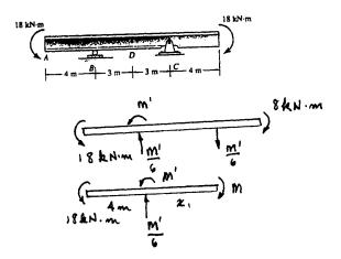
$$\theta_B = \int_0^L M(\frac{\partial M}{\partial M'}) \frac{dx}{EI} = \int_0^6 \frac{(-18)(-\frac{1}{6}x)dx(10^3)}{EI}$$
