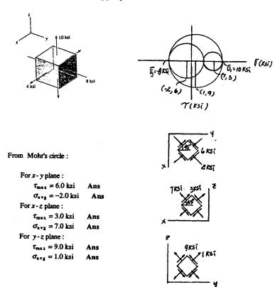
9-91 The stress at a point is shown on the element. Determine the principal stresses and the absolute maximum shear stress.
