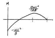
12-106. The loading on a floor beam used in the airplane is shown. Use discontinuity functions and determine the reactions at the supports A and B, and then draw the moment diagram for the beam. The beam is made of aluminum and has a moment of inertia of I = 320 in<sup>4</sup>.
