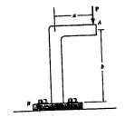
12-98. The rod is pinned at its end A and attached to a torsional spring having a stiffness k, which measures the torque per radian of rotation of the spring. If a force P is always applied perpendicular to the end of the rod, determine the displacement of the force. EI is constant.
