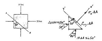
$$\sigma_{x'} \Delta A + 14 \Delta A \sin 50^{\circ} \cos 40^{\circ} + 20 \Delta A \cos 50^{\circ} \cos 50^{\circ} = 0$$
