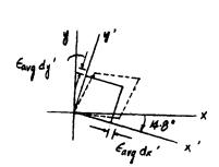
\*10-8 The state of strain at the point on the gear tooth has the components  $\epsilon_x = 520(10^{-6})$ ,  $\epsilon_y = -760(10^{-6})$ .  $\gamma_{xy}$ -750(10-6). Use the strain-transformation equations to determine (a) the in-plane principal strains and (b) the maximum in plane shear strain and average normal strain. In each case specify the orientation of the element and show how the strains deform the element within the x-y plane.
