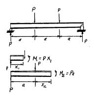
$$U_{i} = \int_{0}^{L} \frac{M^{2} dx}{2EI} = \frac{1}{2EI} \left[ 2 \int_{0}^{a} (Px_{1})^{2} dx_{1} + \int_{0}^{a} (Pa)^{2} dx_{2} \right]$$
