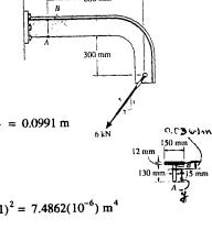
$$\bar{y} = \frac{\Sigma \bar{y} A}{\Sigma A} = \frac{0.065(0.13)(0.015) + 0.136(0.15)(0.012)}{0.13(0.015) + 0.15(0.012)} = 0.0991 \text{ m}$$
