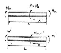
$$\theta_B = \int_0^L M(\frac{\partial M}{\partial M'}) \frac{dx}{EI} = \int_0^L \frac{M_0(1)}{EI} dx$$
