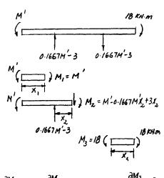
$$\frac{\partial M_1}{\partial M'} = 1 \qquad \frac{\partial M_2}{\partial M'} = 1 - 0.1667x_2 \qquad \frac{\partial M_3}{\partial M'} = 0$$
