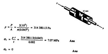
The pressure p is supported by the surface of the pistons in the longitudinal direction.
