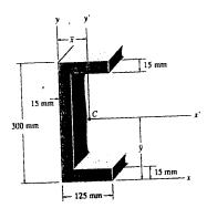
$$\bar{x} = \frac{\Sigma \bar{x}A}{\Sigma A} = \frac{(62.5)(2)(125)(15) + (7.5)(270)(15)}{2(125)(15) + 270(15)} = 33.942 \text{ mm} = 33.9 \text{ mm}$$
