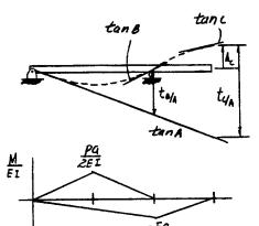
$$t_{B/A} = \frac{1}{2} (\frac{Pa}{2EI})(2a)(a) + \frac{1}{2} (-\frac{Fa}{EI})(2a)(\frac{2}{3}a) = \frac{Pa^3}{2EI} - \frac{2Fa^3}{3EI}$$
