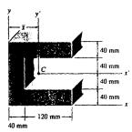
$$\bar{x} = \frac{\Sigma \bar{x}A}{\Sigma A} = \frac{(20)(160)(40) + 2[100(120)(40)]}{160(40) + 2[120(40)]} = 68.0 \text{ mm}$$
