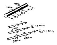
$$U_i = \Sigma \frac{T^2 L}{2JG} = \frac{1}{2JG} [0^2 (0.5) + ((3)(10^3))^2 (0.5) + ((1)(10^3))^2 (0.5)]$$
