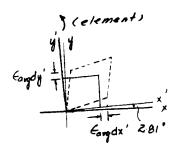
10-29. The 45° strain rosette is mounted on the link of the backhoe. The following readings are obtained from each gauge:  $\epsilon_a = 650(10^{-6})$ ,  $\epsilon_b = -300(10^{-6})$ ,  $\epsilon_c = 480(10^{-6})$ . Determine (a) the in-plane principal strains and (b) the maximum in-plane shear strain and associated average normal strain.
