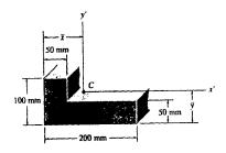
$$\bar{x} = \frac{\Sigma \bar{x}A}{\Sigma A} = \frac{25(50)(50) + 100(50)(200)}{50(50) + (50)(200)} = 85 \text{ mm}$$
