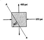
$$\sigma_{x} = -650 \text{ psi} \qquad \sigma_{y} = 400 \text{ psi} \qquad \tau_{xy} = 0 \qquad \theta = 30^{\circ}$$
