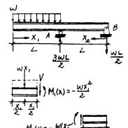
$$v_1 = \frac{w}{24EI}(-x_1^4 + 8L^3x_1 - 7L^4)$$
