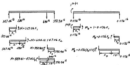
$$\begin{aligned} \mathbf{1} \cdot \theta_A &= \int_0^L \frac{m_\theta M}{EI} dx \\ \theta_A &= \frac{1}{EI} [\int_0^2 (1 - 0.1176x_1)(327.06x_1) dx_1 + \int_0^{1.5} (0.1176x_3)(592.94x_3) dx_3 \\ &+ \int_0^5 0.1176(x_4 + 1.5)(889.41 - 47.06x_4) dx_4 ] \\ &= \frac{2387.53 \text{ lb} \cdot \text{ft}^2}{EI} = \frac{2387.53(12^2)}{29(10^6)(\frac{\pi}{4})(0.75^4)} = 0.0477 \text{ rad} = 2.73^\circ \end{aligned}$$
