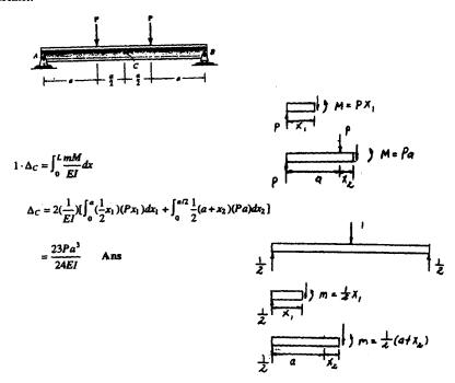
\*14-88 Determine the displacement at point C. EI is constant.
