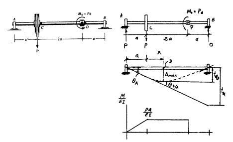
$$t_{B/A} = \frac{1}{2}(\frac{Pa}{EI})(a)(3a + \frac{a}{3}) + (\frac{Pa}{EI})(2a)(a + a) = \frac{17Pa^3}{3EI}$$
