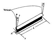
$$y_{\text{max}} = \frac{P \cos \theta L^3}{3EI_x}; \qquad x_{\text{max}} = \frac{P \sin \theta L^3}{3EI_y}$$
