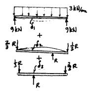
12-126 Determine the reactions at A and B. Assume the support at A only exerts a moment on the beam. El is con-
