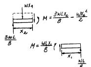
$$U_{i} = \int_{0}^{L} \frac{M^{2} dx}{2EI} = \frac{1}{2EI} \left[ \int_{0}^{L/2} \left( \frac{3wLx_{2}}{8} - \frac{wx_{2}^{2}}{2} \right)^{2} dx_{2} + \int_{0}^{L/2} \left( \frac{wLx_{1}}{8} \right)^{2} dx_{1} \right]$$
