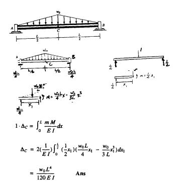
14-111 Determine the slope of the shaft at the bearing support A, EI is constant.
