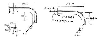
$$\bar{y} = \frac{\Sigma \bar{y} A}{\Sigma A} = \frac{0.065(0.13)(0.015) + 0.136(0.15)(0.012)}{0.13(0.015) + 0.15(0.012)} = 0.0991 \text{ m}$$
