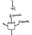
**8-75.** The crowbar is used to pull out the nail at A. If a force of 8 lb is required, determine the stress components in the bar at points D and E. Show the results on a differential volume element located at each of these points. The bar has a circular cross section with a diameter of 0.5 in. No slipping occurs at B.
