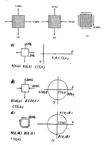
9-79 A point on a thin plate is subjected to two successive states of stress as shown. Determine the resulting state of stress with reference to an element oriented as shown on the right.
