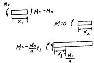
$$U_{i} = \int_{0}^{L} \frac{M^{2} dx}{2EI} = \frac{1}{2EI} \left[ \int_{0}^{a} (-M_{0})^{2} dx_{1} + \int_{0}^{a} (0) dx_{2} + \int_{0}^{a} (-\frac{M_{0}}{a} x_{3})^{2} dx_{3} \right]$$
