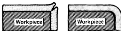
Fig. 9 Effect of sharp and round corners on the continuity of a ceramic coating
