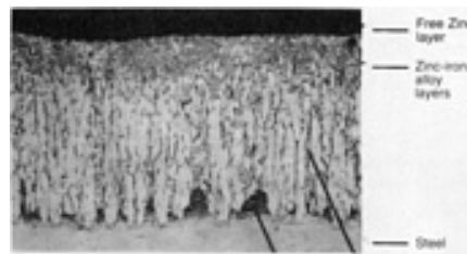
Fig. 7 Photomicrograph of a galvanized coating on a steel containing 0.40% Si. 250×
