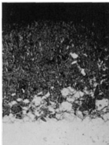
Fig. 8 Observable diffusion zone on the unetched (white) portion of an ion-nitrided 416 stainless steel. Nital etched. 500x
