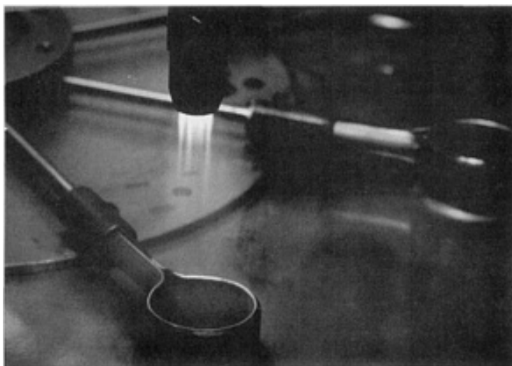
Fig. 2 Flame impingement on the button sample in a thermal fatigue test rig
