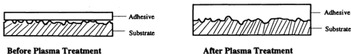
Fig. 3 Schematic of ablation, or microroughening, of the surface layer of a polymer substrate by plasma surface modification. Microroughening increases the area of contact between an adhesive and a substrate to strengthen the bond.
