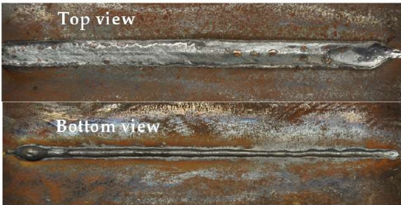
Figure 7. A514 sample achieved by 3.8 kW laser and 159A×30.5V GMAW with a welding speed of 12 mm/s and 8-mm stand-off distance between the laser and arc
