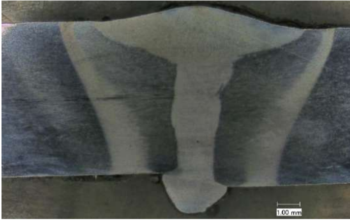
Figure 8. Cross-sectional view of A514 weld sample achieved by 3.8 kW laser and 159A×30.5V GMAW with a welding speed of 12 mm/s and 8-mm stand-off distance between the laser and arc
