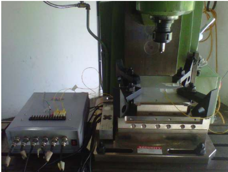
Figure 1. Friction stir welding experimental set up [5].
