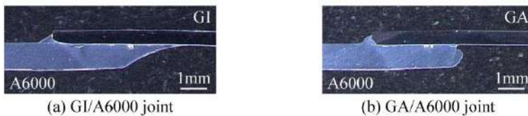
Figure 8. Macro cross-section of GI/A6000 and GA/A6000 Laser Roll Welded joints
