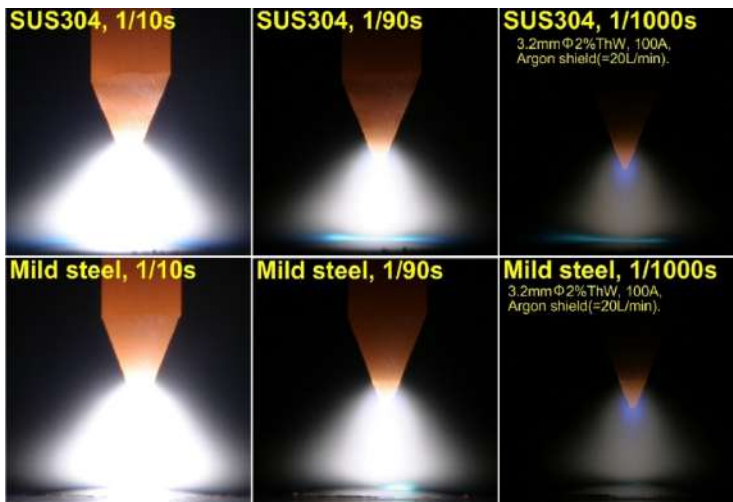
Figure 6. Example of argon arc image on metal plates.
