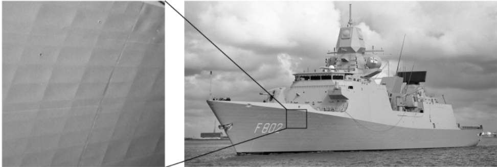
Figure 8. Ship hull defect due to distortion (van der Aa, 2007) .
