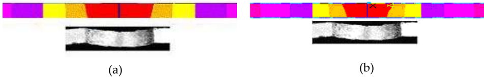
Figure 12. Experimental & simulated fusion boundary fitting: (a) double ellipsoid; (b) gaussian distribution;
