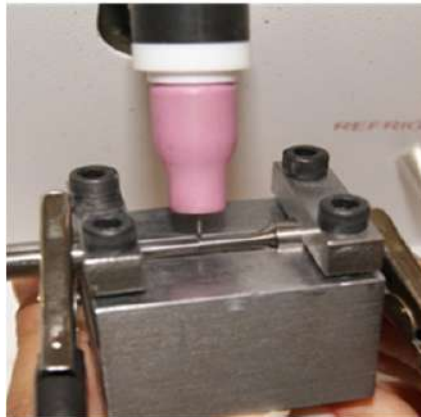
Figure 4. Ceramic torch, with tungsten electrode, positioned over the sample.
