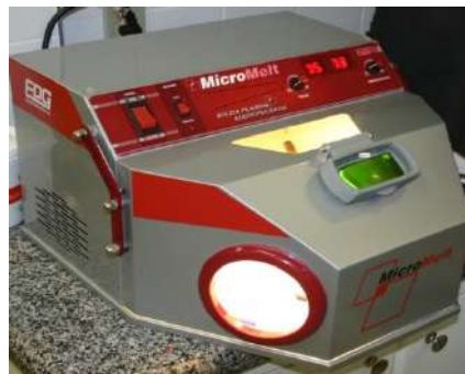
Figure 5. Plasma welding machine for Dentistry.
