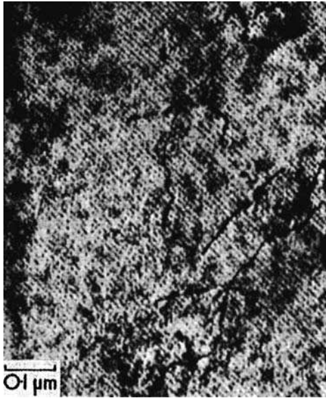
Fig. 4.15 Fe-0.75V-0.15C transformed 5 min at 725°C. Interphase precipitation of VC in ferrite (courtesy of Batte). Thin-foil electron micrograph.
