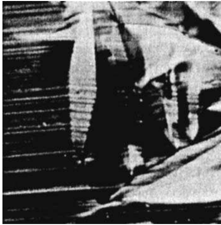
Fig. 5.4 Fe–30.5Ni–0.3C wt% illustrating the displacement of surface scratches by the martensitic shear. Nomarski interference contrast, \times 650 .
