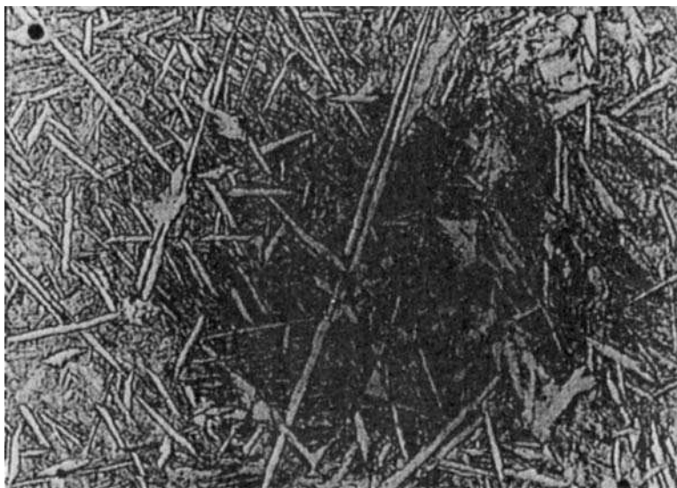
Fig. 7.2 Replica transmission electron micrograph of acicular ferrite plates in martensite matrix, in a steel weld deposit which was partially transformed and quenched (courtesy of Barritte).
