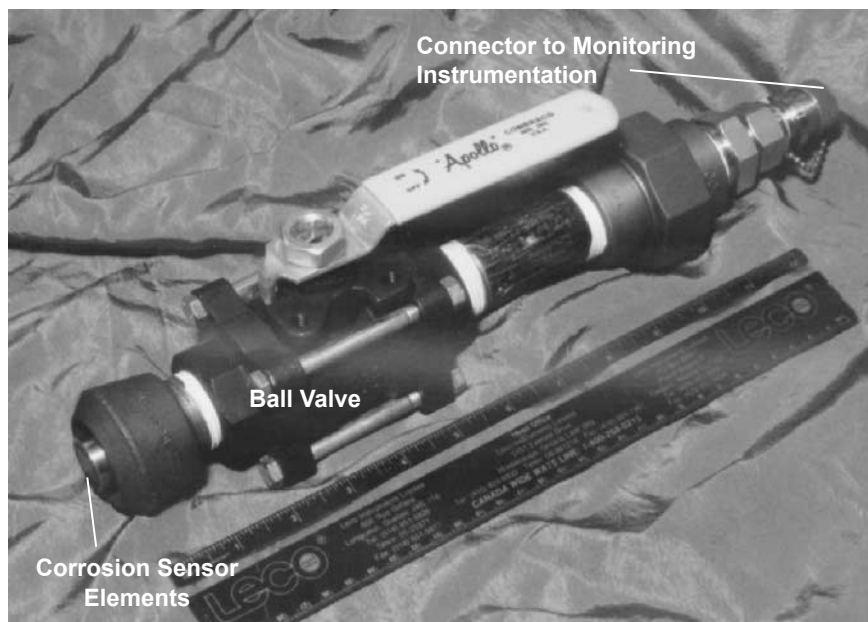
Figure 6.25 Corrosion sensor and access fitting used for thin-film corrosion monitoring.
