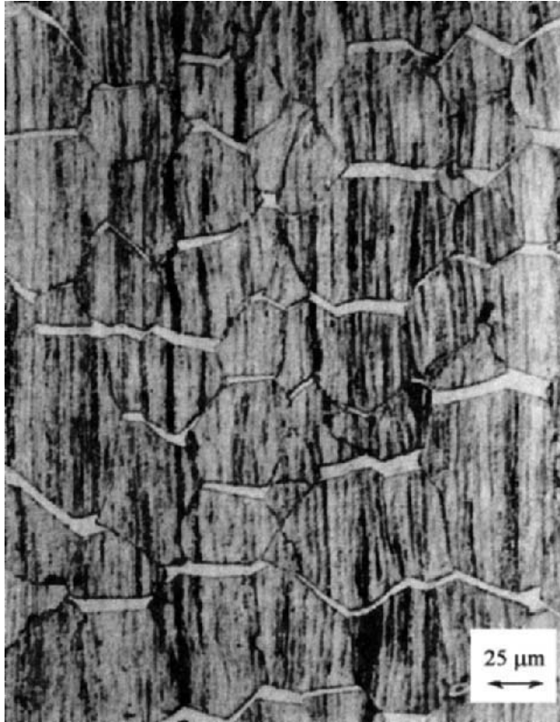
Figure 48. Denuded zones formed perpendicular to the tensile direction in a hydrated Mg-0.5%Zr alloy at 400°C and 2.1 MPa [262].
