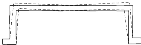
Figure 8.7 Distortion of an open-sided box casting during cooling as a result of uneven mould constraint.
