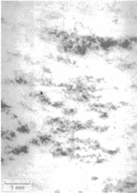
Figure 7.24 Radiograph of interdendritic porosity in a carbon steel (Campbell 1969).
