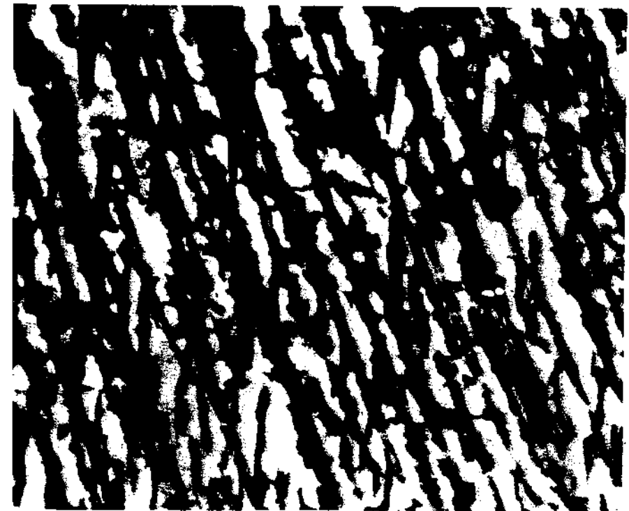
Fig. 6.25 \epsilon -carbide (dark) precipitated from martensite in Fe-24 Ni-0.5 C after 30 min at 250 °C. Thin foil electron micrograph ( \times 90\,000 ). (After G.R. Speich in Metals Handbook , 8th edn. Vol. 8, American Society for Metals, 1973, p. 202.)
