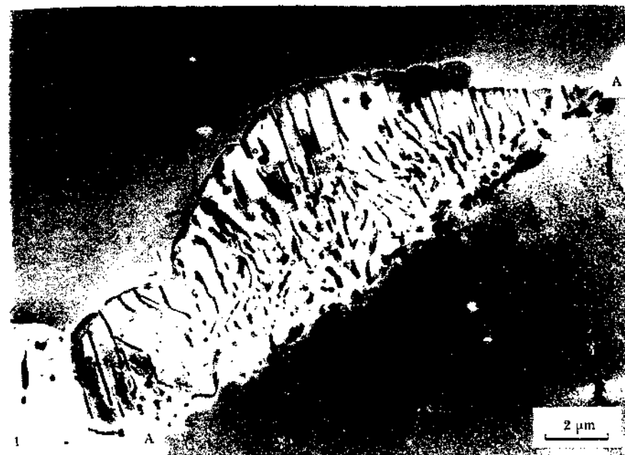
Fig. 5.51 Cellular precipitation of Mg_{17}Al_{12} in an Mg-9 at% Al alloy solution treated and aged 1 h at 220 °C followed by 2 min at 310 °C. Some general Mg_{17}Al_{12} precipitation has also occurred on dislocations within the grains.
