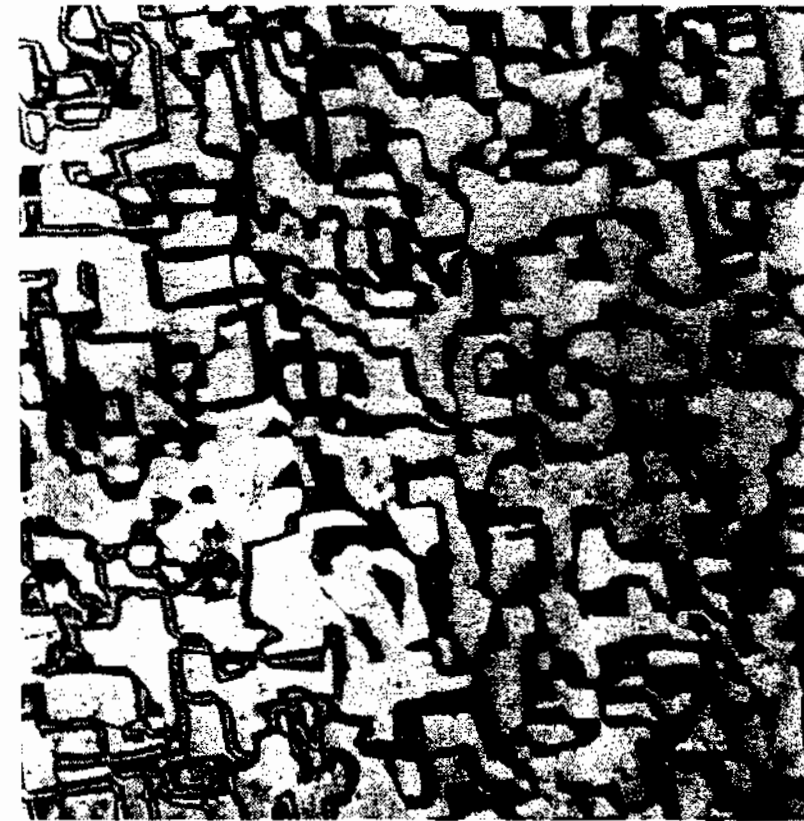
Fig. 5.86 APBs in ordered \text{Cu}_3\text{Au} . Thin-foil electron micrograph \times 53\,000 . Note that due to the method of imaging about one third of the APBs are invisible. (After M.J. Marcinkowski in Metals Handbook , 8th edn., Vol. 8. American Society for Metals, 1973, p. 205.)
