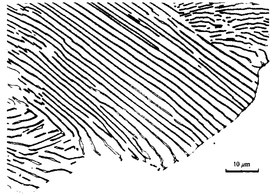
Fig. 5.55 A pearlite colony advancing into an austenite grain. (After L.S. Darken and R.M. Fisher in Decomposition of Austenite by Diffusional Processes , V.F. Zackay and H.I. Aaronson (Eds.), by permission of The Metallurgical Society of AIME.
