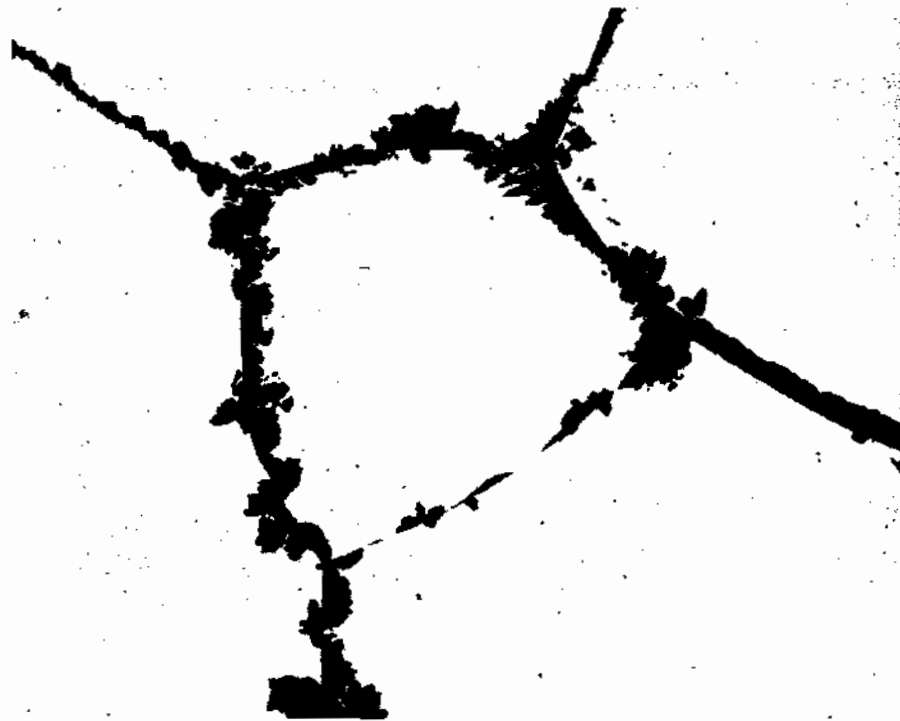
Fig. 5.56 A partially transformed eutectoid steel. Pearlite has nucleated on grain boundaries and inclusions ( \times 100 ). (After J.W. Cahn and W.C. Hagel in Decomposition of Austenite by Diffusional Processes , V.F. Zackay and H.I. Aaronson (Eds.), 1962, by permission of The Metallurgical Society of AIME.)
