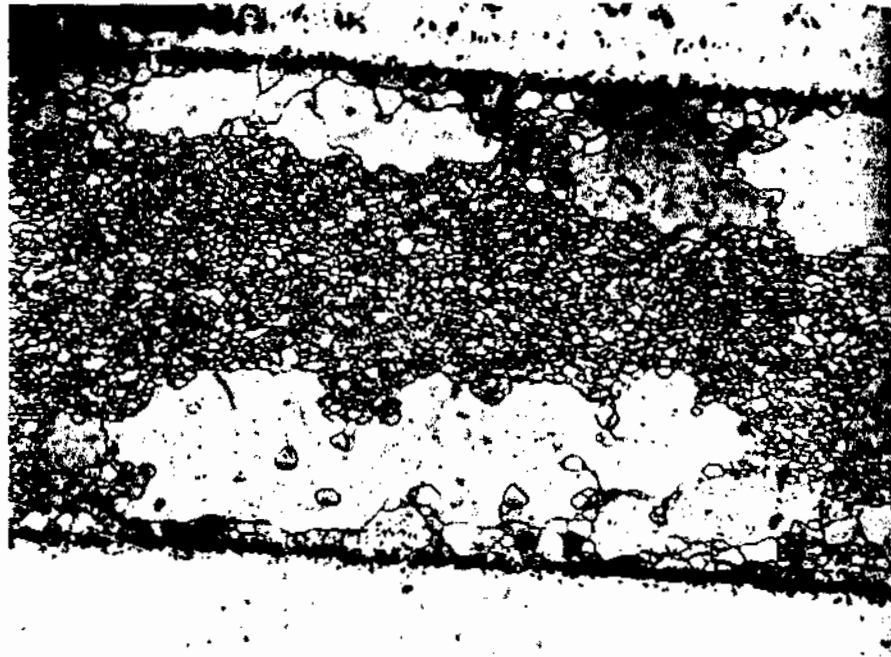
Fig. 3.29 Optical micrograph ( \times 130 ) showing abnormal grain growth in a fine-grained steel containing 0.4 wt% carbon. The matrix grains are prevented from growing by a fine dispersion of unresolved carbide particles. (After D.T. Gawne and G.T. Higgins, Journal of the Iron and Steel Institute , 209 (1971), 562.)
