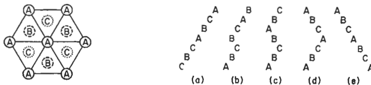
Fig. 32. Planar view of atomic positions and stacking sequences for: (a) perfect fcc crystal; (b) intrinsic fault; (c) extrinsic fault; (d) twin fault; (e) twin crystal. (After JOHNSON [1963].)
