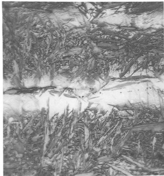
Fig. 5.34(b) Nonmetallic inclusions and banding in a heavily microsegregated 1% C alloy steel sample. Retained austenite, light
