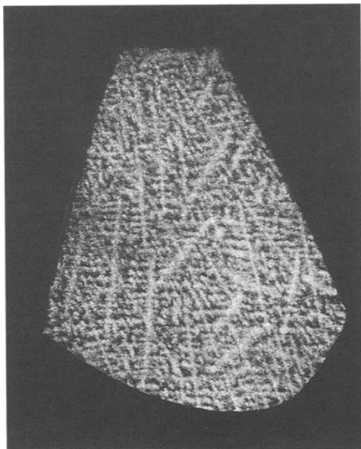
Fig. 5.28 Dendritic microsegregation in a fractured gear tooth. 2x
