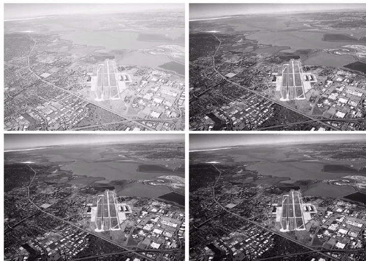
a b c d FIGURE 3.9 (a) Aerial image. (b)–(d) Results of applying the transformation in Eq. (3.2-3) with c = 1 and \gamma = 3.0, 4.0, and 5.0, respectively. (Original image for this example courtesy of NASA.)
