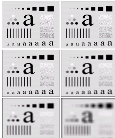
FIGURE 3.35 (a) Original image, of size 500 \times 500 pixels. (b)–(f) Results of smoothing with square averaging filter masks of sizes n = 3, 5, 9, 15, and 35 , respectively. The black squares at the top are of sizes 3, 5, 9, 15, 25, 35, 45, and 55 pixels, respectively; their borders are 25 pixels apart. The letters at the bottom range in size from 10 to 24 points, in increments of 2 points; the large letter at the top is 60 points. The vertical bars are 5 pixels wide and 100 pixels high; their separation is 20 pixels. The diameter of the circles is 25 pixels, and their borders are 15 pixels apart; their gray levels range from 0% to 100% black in increments of 20%. The background of the image is 10% black. The noisy rectangles are of size 50 \times 120 pixels.
