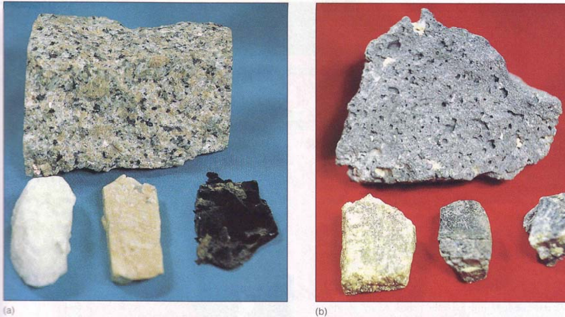
(a) (b) FIGURE 2.20 The mineral composition of two igneous rocks. (a) Granite contains mostly quartz (left), potassium feldspar (center) and small amounts of biotite (right). (b) Basalt is made up of some olivine (left), but contains mostly pyroxene (center), and calcium plagioclase (right). The sizes of minerals in these rocks depends on how rapidly they cooled from molten rock material (see Chapter 10). (Photos courtesy of Sue Monroe.)
