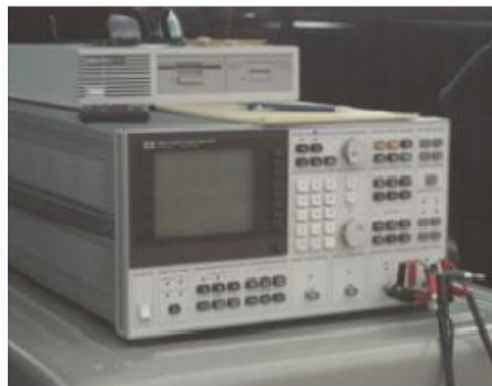
Figure 5-29. Spectrum Analyzer and Data Logging Equipment for SASW.
