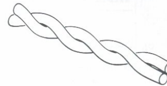
Twisted bar (round sections) Isteg steel
