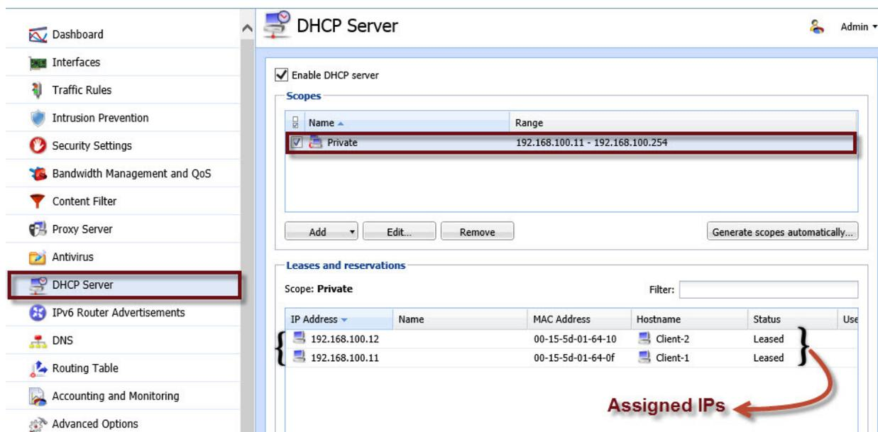
The screenshot shows the DHCP Server configuration interface. The left sidebar has 'DHCP Server' highlighted. The main panel shows 'Enable DHCP server' checked. Under 'Scopes', there is a table with one entry: 'Private' with range '192.168.100.11 - 192.168.100.254'. Below that are 'Add', 'Edit...', and 'Remove' buttons, and a 'Generate scopes automatically...' button. Under 'Leases and reservations', the scope is set to 'Private'. A table shows the following data:
