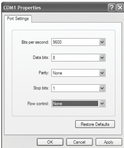
Figure 4-3 PC Settings to Connect to a Router or Switch
