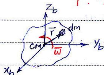
$$d\bar{H} = \bar{r} \times dm \times \bar{w} \times \bar{r}$$
