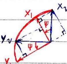
$$\Rightarrow \begin{Bmatrix} X_1 \\ Y_1 \\ Z_1 \end{Bmatrix} = \begin{Bmatrix} \cos \psi & \sin \psi & 0 \\ -\sin \psi & \cos \psi & 0 \\ 0 & 0 & 1 \end{Bmatrix} \begin{Bmatrix} X_v \\ Y_v \\ Z_v \end{Bmatrix}$$
