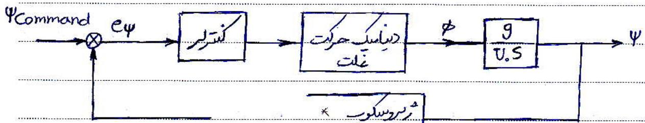
$$\phi = \frac{U_0^2}{R \cdot g} = \frac{(R \cdot \dot{\psi} U_0)}{R \cdot g} = \frac{U_0 \cdot \dot{\psi}}{g} \quad \dot{\psi} = \frac{g}{U_0} \phi \quad \psi = \frac{g}{U \cdot S} \phi$$
