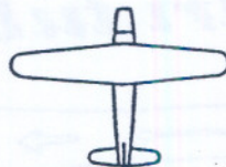
TAPERED LEADING AND TRAILING EDGES
