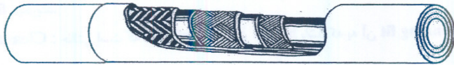
MIL-H-8788 has two steel wire braids for reinforcement and is covered with a smooth outer cover.
