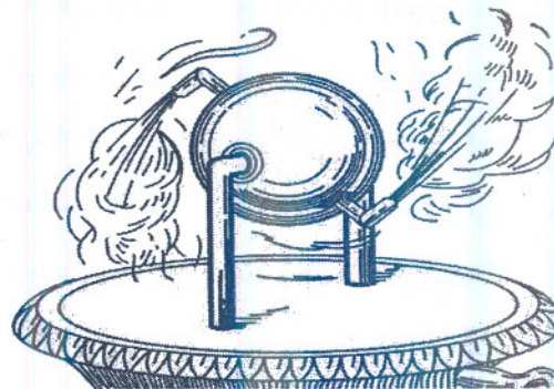
A garden water sprinkler rotated by the reaction of the water jets.
