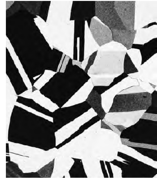
Photomicrograph of Brass Alloy
