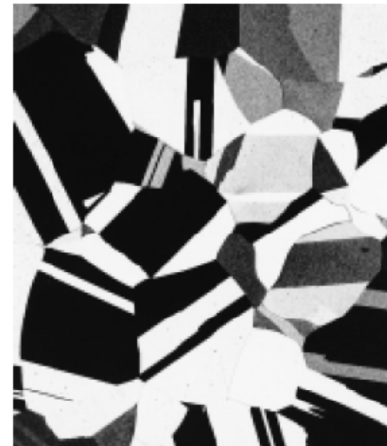
Grain growth 10 min at 700C
