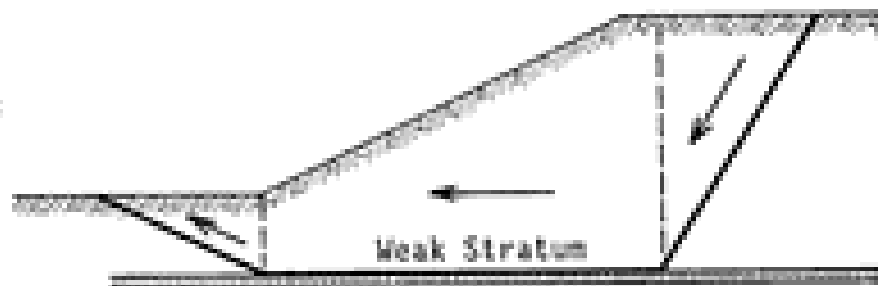
Sliding Block Failure
