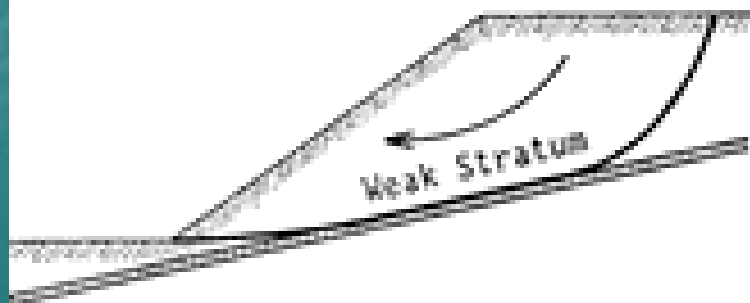
Non-Circular Failure Surface
